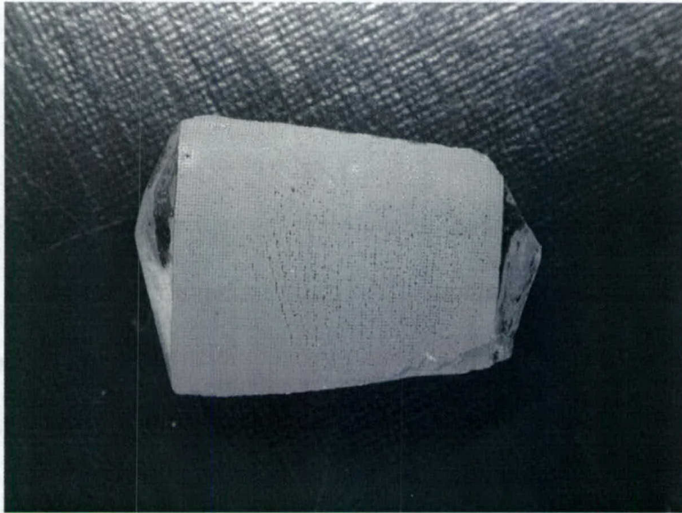
Figure 18: The picture of the barium-oxide doped sample with a 120 \mu\text{m} -pitch dot array sintered at 1725 ^{\circ}\text{C} for 0 minutes in vacuum.
