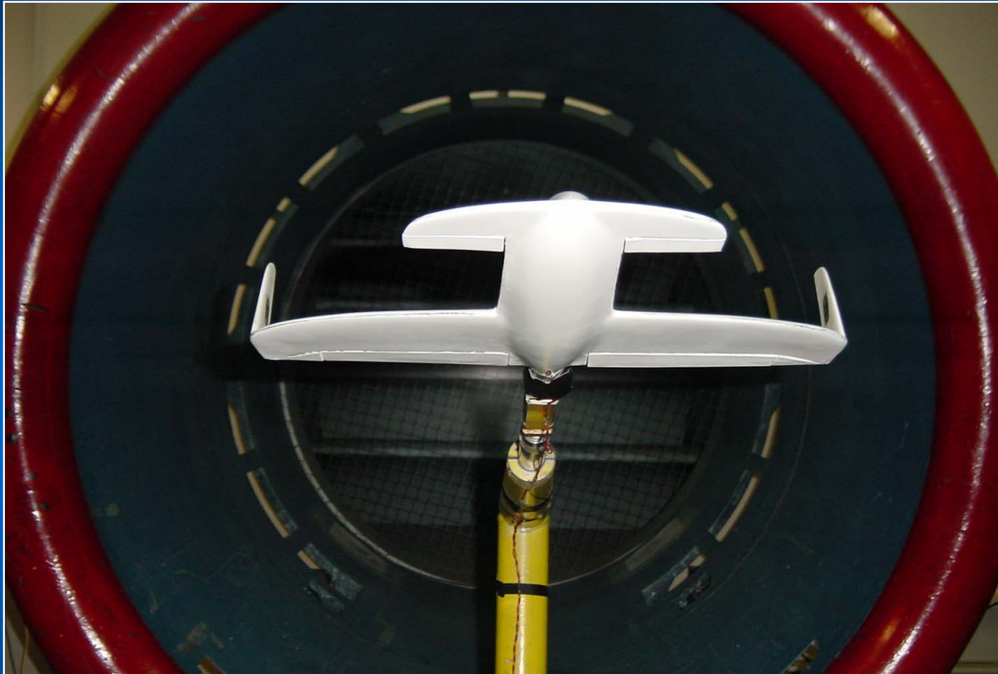
CAROLO during wind tunnel tests at the Institute of Fluid Dynamics, Technical University of Braunschweig
