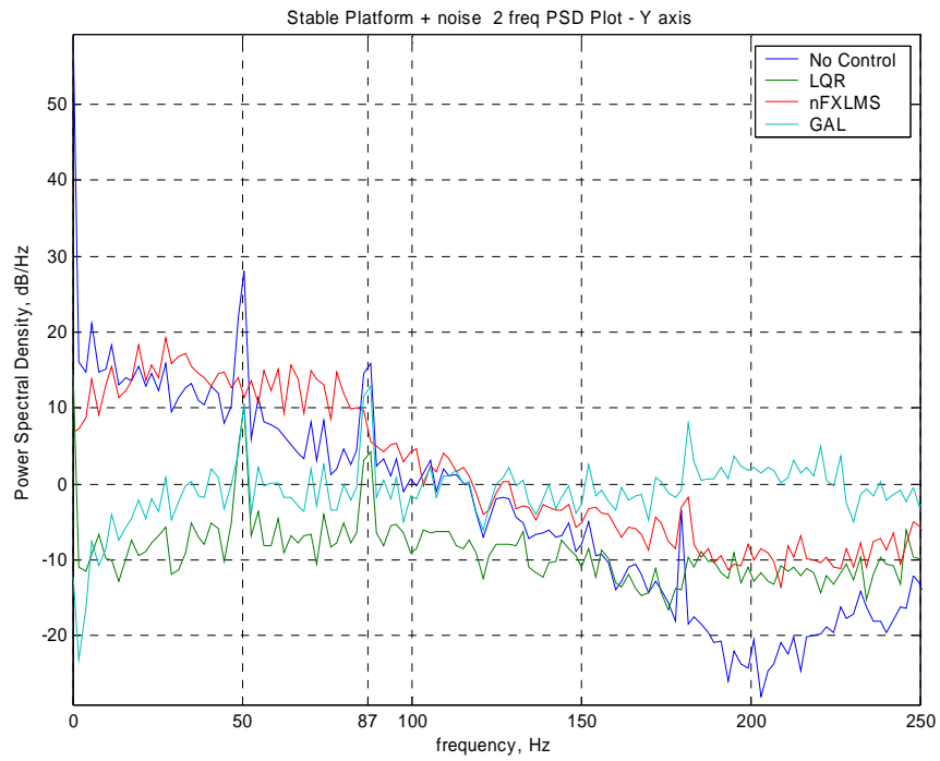
Figure 98 PSD Case 2, DFSM narrowband disturbance plus 200 Hz noise
