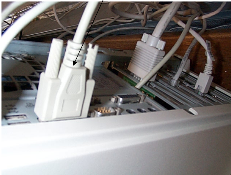
Serial cable on the back of the PC
