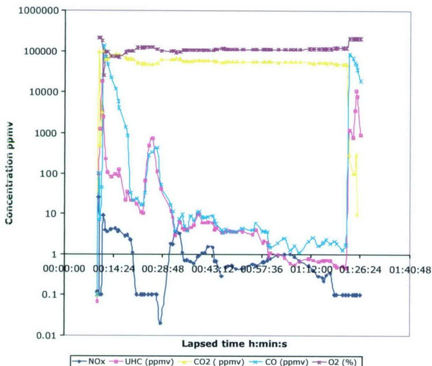
Figure 23 Single Trials Point Record for Gaseous Emissions, on CH<sub>4</sub> at 1100kPa and 450K Inlet Conditions as for Figure 18, ER=0.5.
