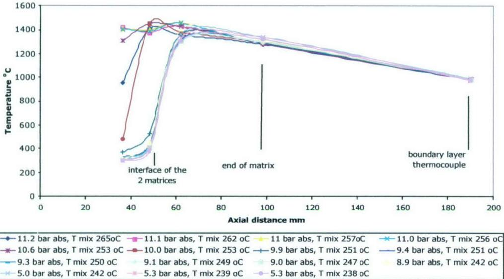
Figure 20 Alteration of Stable Operating Condition with Pressure.
