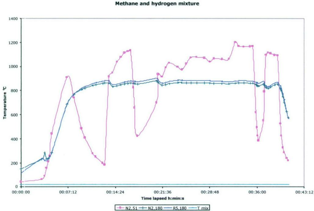
Figure 15 Exit Gas & 1 Matrix Temperature from Combustion of  $\text{CH}_4/\text{H}_2$  Mixture in the 3-matrix Arrangement, showing large Excursions at the Fine/Coarse Pore Interface. Combined Hydrogen/Methane ER range 0.6 – 0.55.
