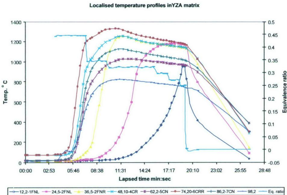
Figure 29 Weak Extinction, indicated by In-matrix Temperature Measurement.
