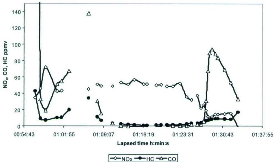
Figure 22 Emissions at Ambient Entry Temperature and 1000kPa; Conditions as Figure 17.
