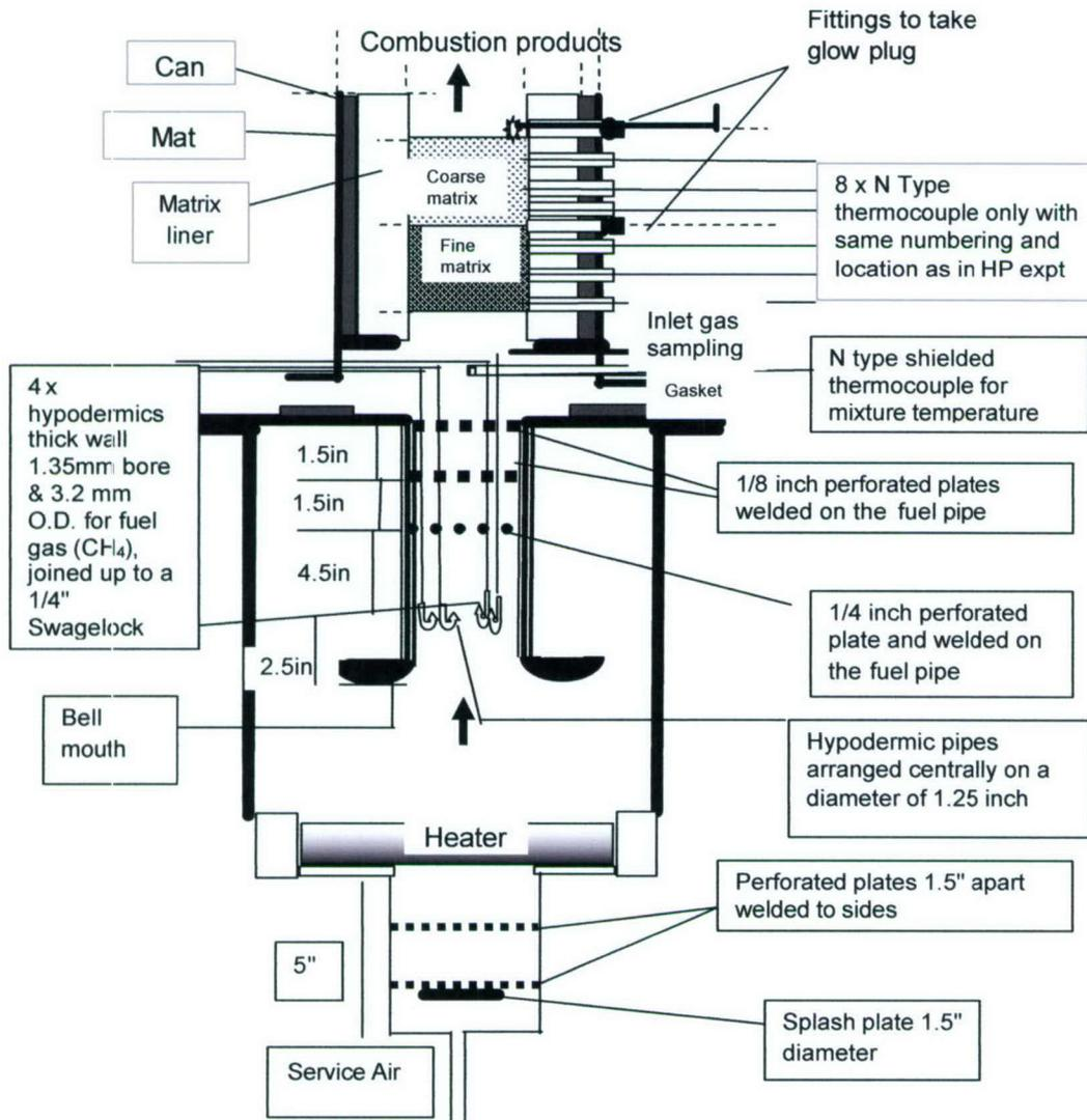
Figure 9 Layout of the Atmospheric Ignition Experiment
