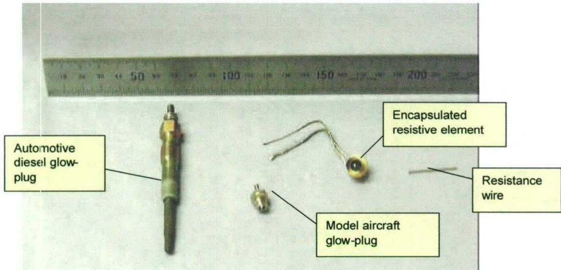
Figure 10 Ignition Devices Trialed.
