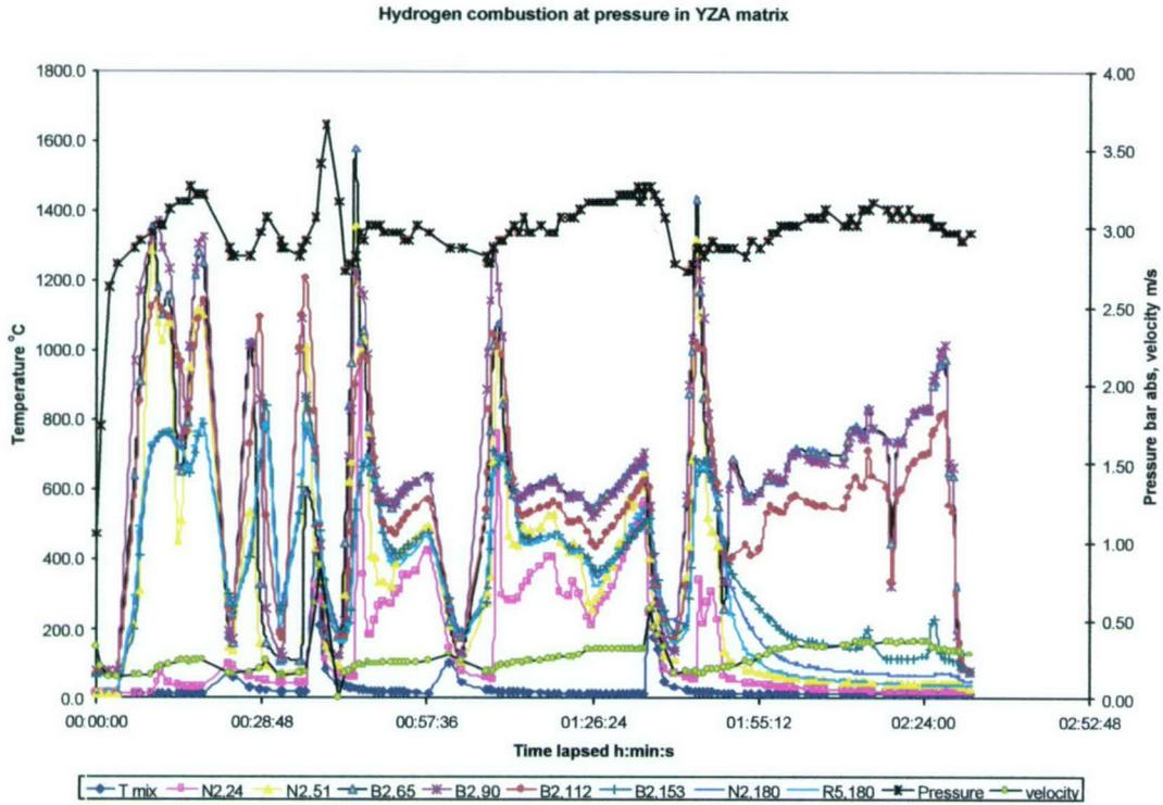
Figure 27 Temperature Profiles of Hydrogen Combustion at 300 kPa.
