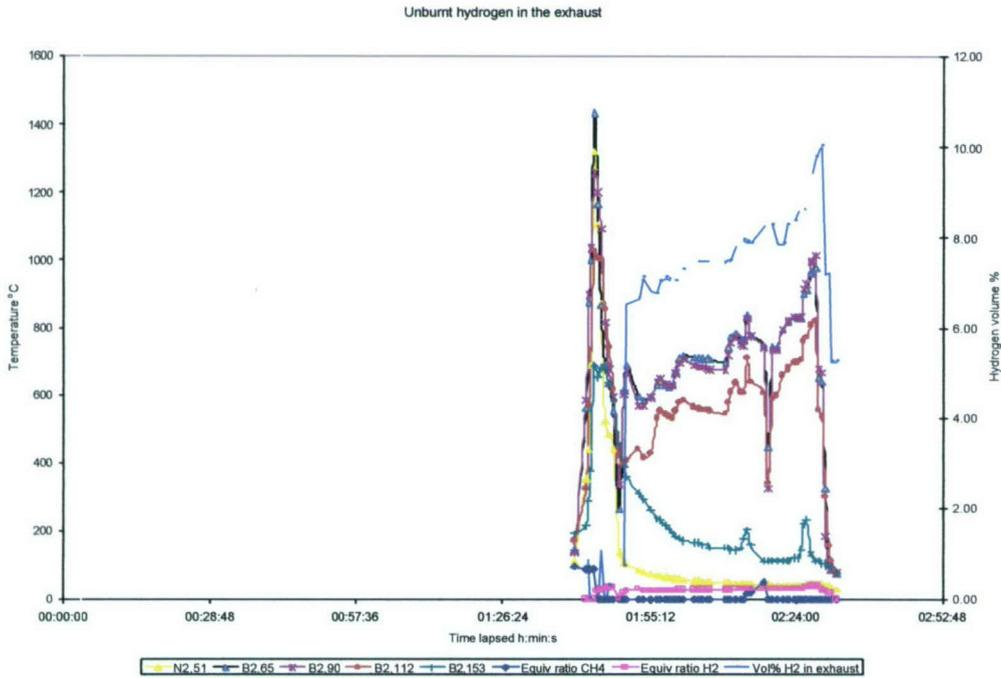
Figure 28 Unburned Hydrogen Remaining in the Exhaust at 300 kPa.
