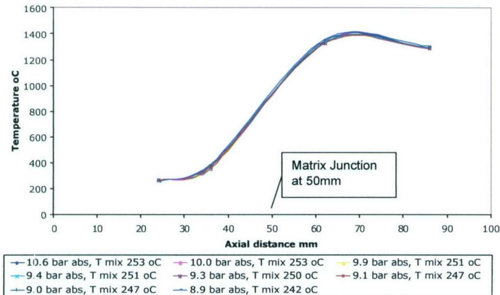
Figure 19 Axial Temperature Profile along the Combustor.
