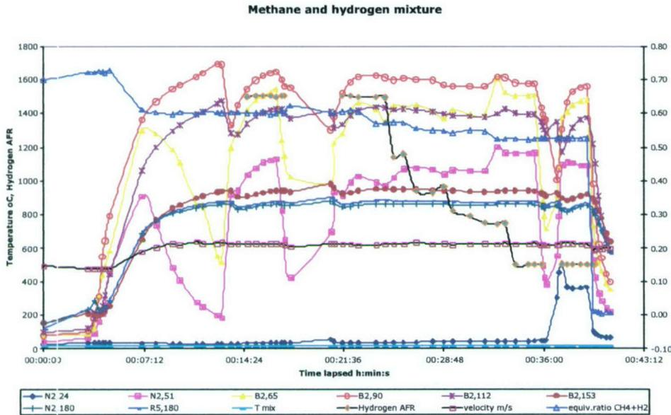
Figure 24 Temperature profiles of combustion of CH<sub>4</sub>/H<sub>2</sub> mixture in the 3-matrix arrangement.
