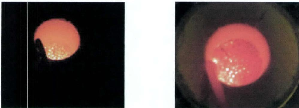
Figure 36 Visible Images of the PMB, showing Structure Effects, left at High ER (~0.4) and right at low ER (~0.25).
