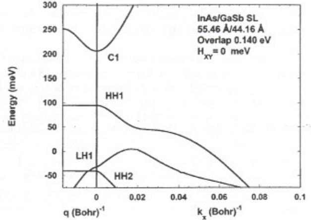
FIG. 1. The band structure of a test InAs/GaSb superlattice with 44.16 Å GaSb/55.46 Å InAs without IF effects using the standard  $8 \times 8$  EFA (Ref. 32). The zero of energy is at the CB edge of bulk InAs.
