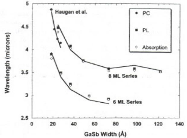
FIG. 4. Collected results of the variable GaSb width studies listed in Tables V, VII, and VIII, where the solid curves are calculated with the modified EFA and the experimental data are from Haugan *et al.* (Ref. 56), Ongstad *et al.* (Ref. 21), and Kaspi *et al.* (Ref. 23).
