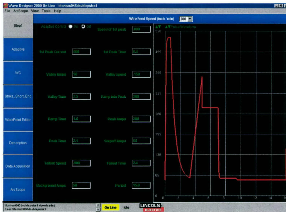
Figure 5. Waveform Used to Effect Proper Transfer During the Pulsed GMAW Tests During Phase I. This pulse form is an optimized sequence for titanium. This waveform cannot currently be varied in response to weld conditions. In Phase II, we will dynamically change the waveform to control the weld process.
