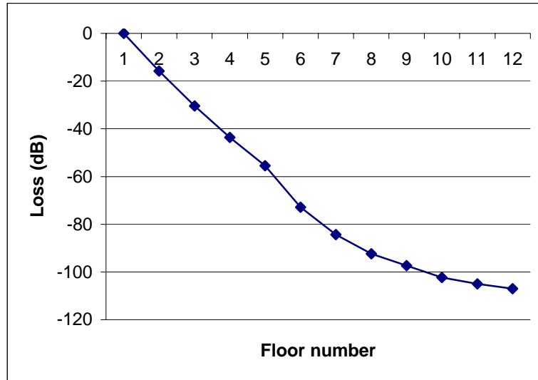
Figure 59. Loss between floors for a high-fidelity building (antenna in the first floor, transmit power 1 W)
