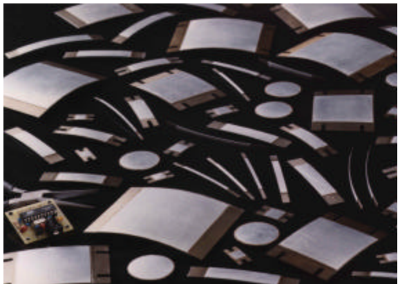
Figure 4. Typical Thunder shapes and sizes
