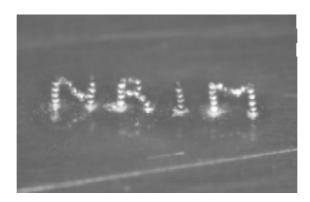
Fig.1 Characters "N", "R", "I" and "M" composed of gold particles
