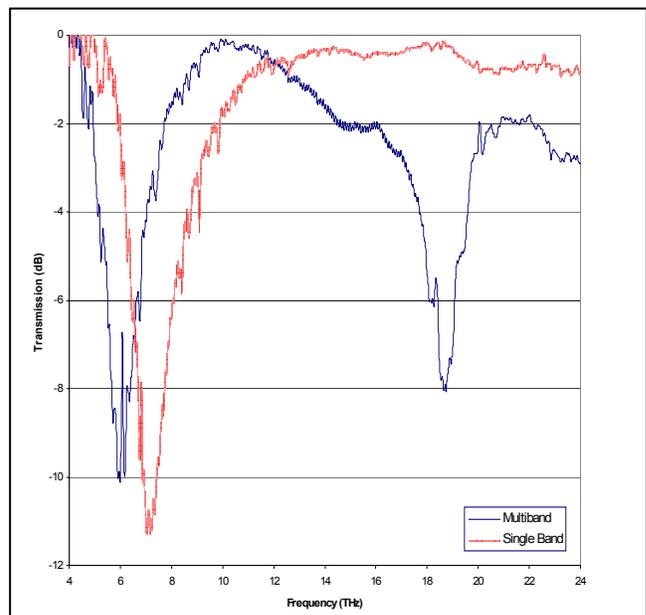
**Fig. 4** Comparison of multiband and single band transmission spectra of cross dipole FSSs with 4  $\mu\text{m}$  polyimide substrate. The primary resonance of the multiband FSS is shifted to a lower frequency than the single band resonance despite identical dimensions. This is because the crossbars of the secondary cross dipoles in the fractal case load the primary crosses, making them electrically longer than their physical size.
