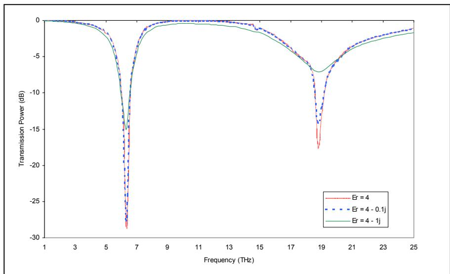
**Fig. 5** A comparison of simulations with different amounts of dielectric loss. The dotted red line is the ideal case with no dielectric loss. The dashed blue line has a small amount of loss, while the solid green line has ten times the amount of loss as the second case. With added loss, the resonances lose depth, and the secondary resonance broadens significantly.
