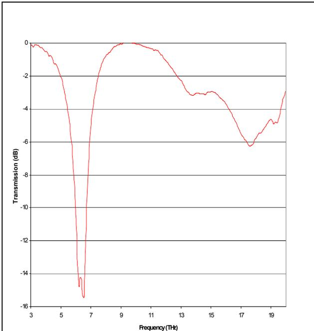
**Fig. 3** Measured transmission spectrum of a FSS on a 200 nm silicon nitride substrate with primary and secondary cross lengths of 17 and 7  $\mu\text{m}$  respectively. The primary resonance is  $-15.3 \text{ dB}$  centered at 6.4 GHz while the secondary resonance is  $-6.2 \text{ dB}$  centered at 17.5 GHz.
