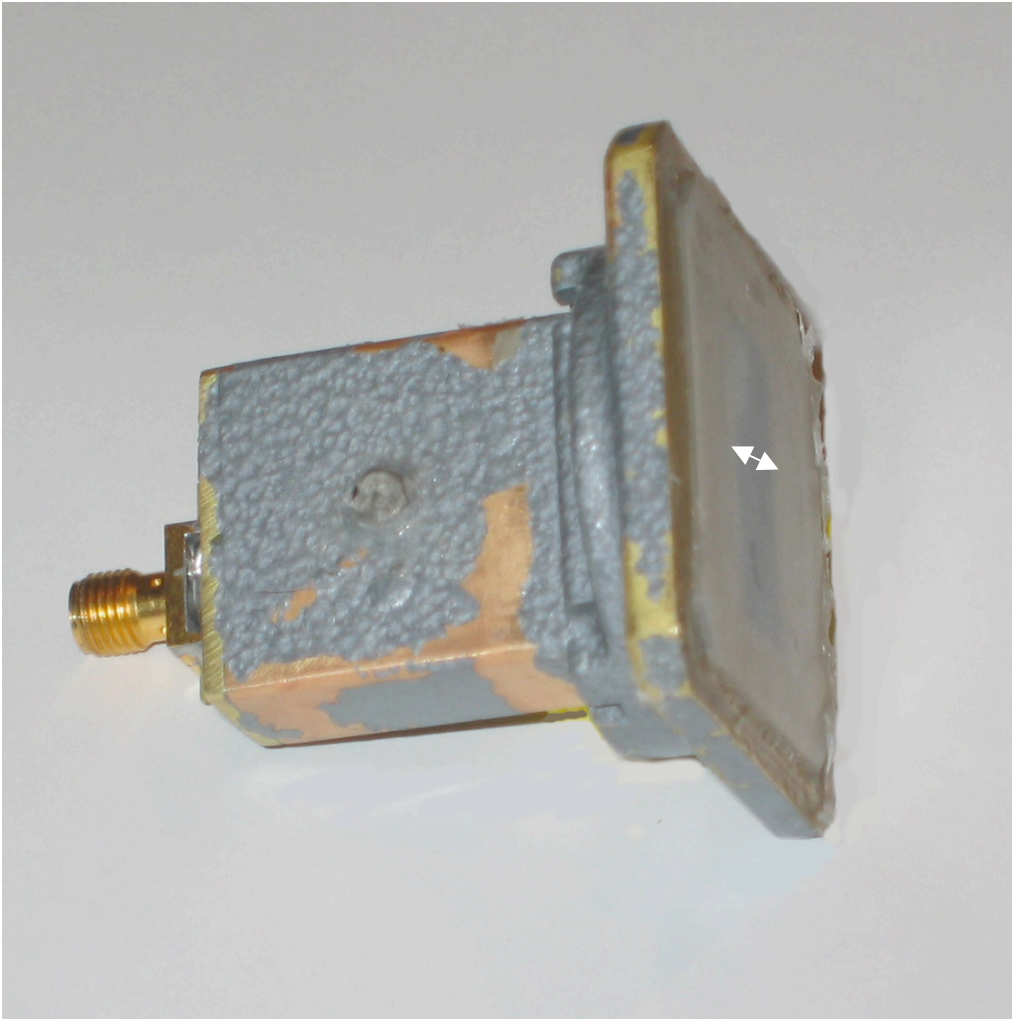
Fig S-2 A rectangular waveguide antenna matched to body tissue using acetone as the dielectric fluid. The arrow shows the direction of the E-field in the transmitted EM wave. This antenna can be used in monostatic mode as well as in bistatic mode, and it preserves polarization. The transverse dimension of the waveguide, also indicated by the double arrow under the plastic cover is about 0.5 inches. This dimension defines the narrowest EM wave beam-width. It was used to define target locations along the neck vertical dimension. Antenna produced by Cyberdynamics Corp, Palo Alto, under license from SNH Instruments LLC.
