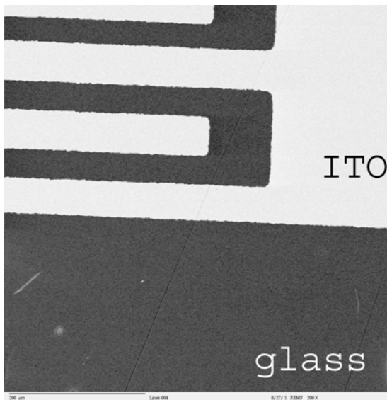
Figures 18, 19. Microstructure of ITO lines (2 is Second Electron Image; 3 is back-scattered Electron image)
