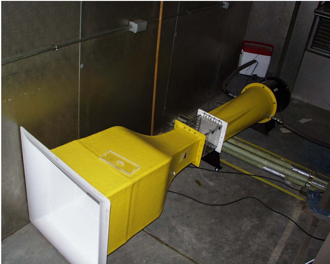
Figure 20. The icing wind tunnel in a cold room.
