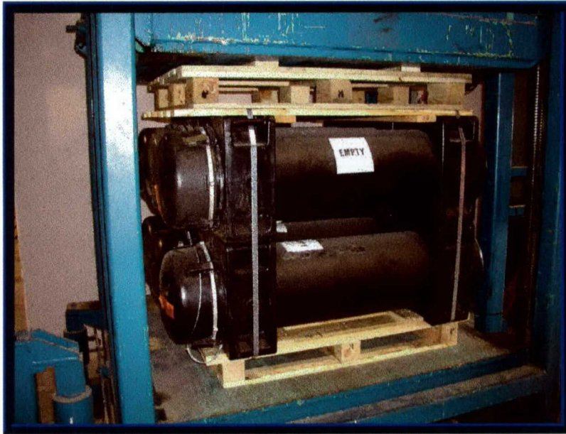
Photo 5. Test Setup for Stacking Test.
