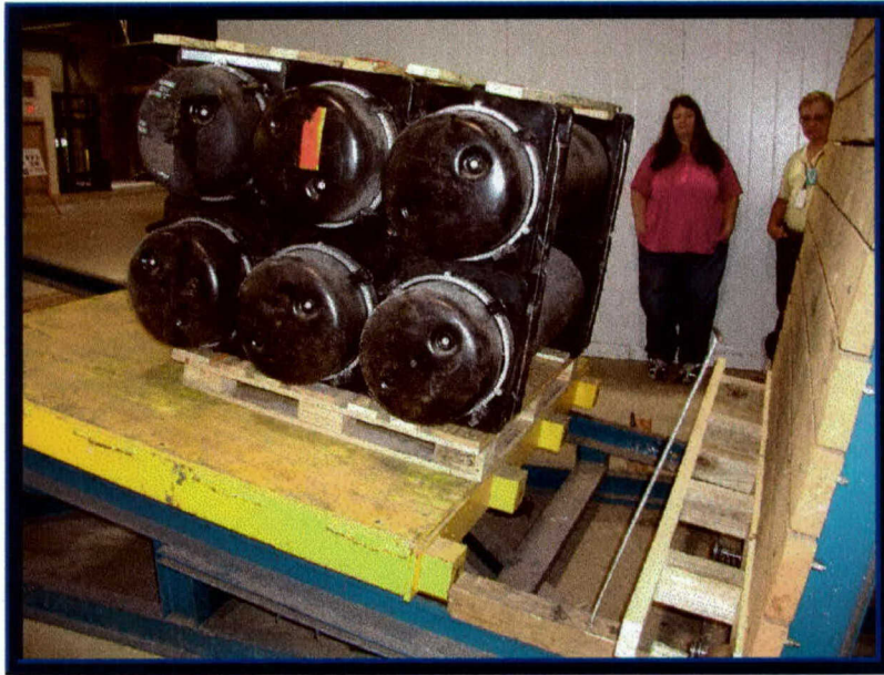
Photo 8. Test Setup for Incline-Impact Testing.
