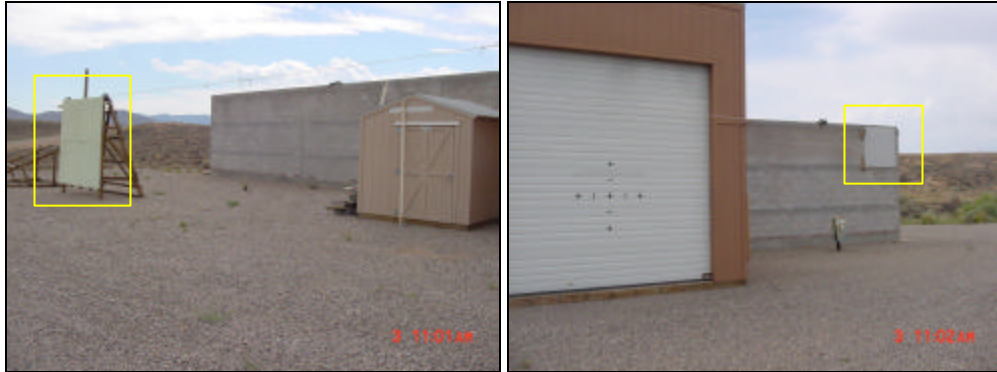
Figure 11. Photographs of left and right sides of the 2KS site, showing the blueboard target (left, 8' x 8') and flame-sprayed aluminum (right, 4' x 4') calibration targets.
