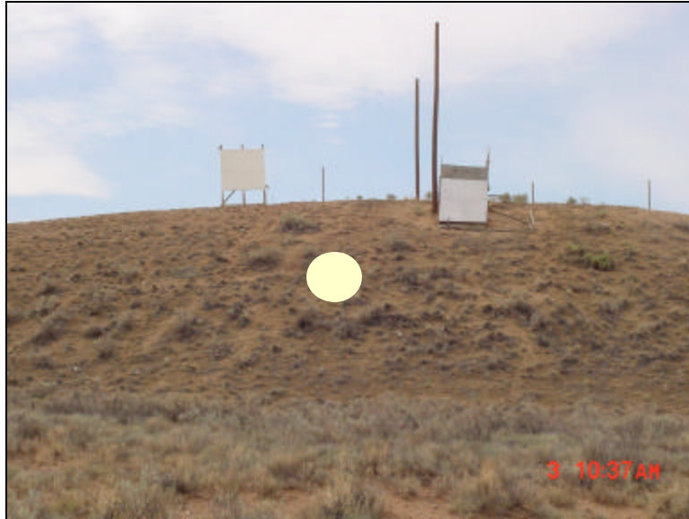
Figure 13. Photograph of 7KS target site, showing aluminum (right) and plywood (left) calibration/pointing target boards and approximate berm illumination area (yellow circle, not exactly to scale).
