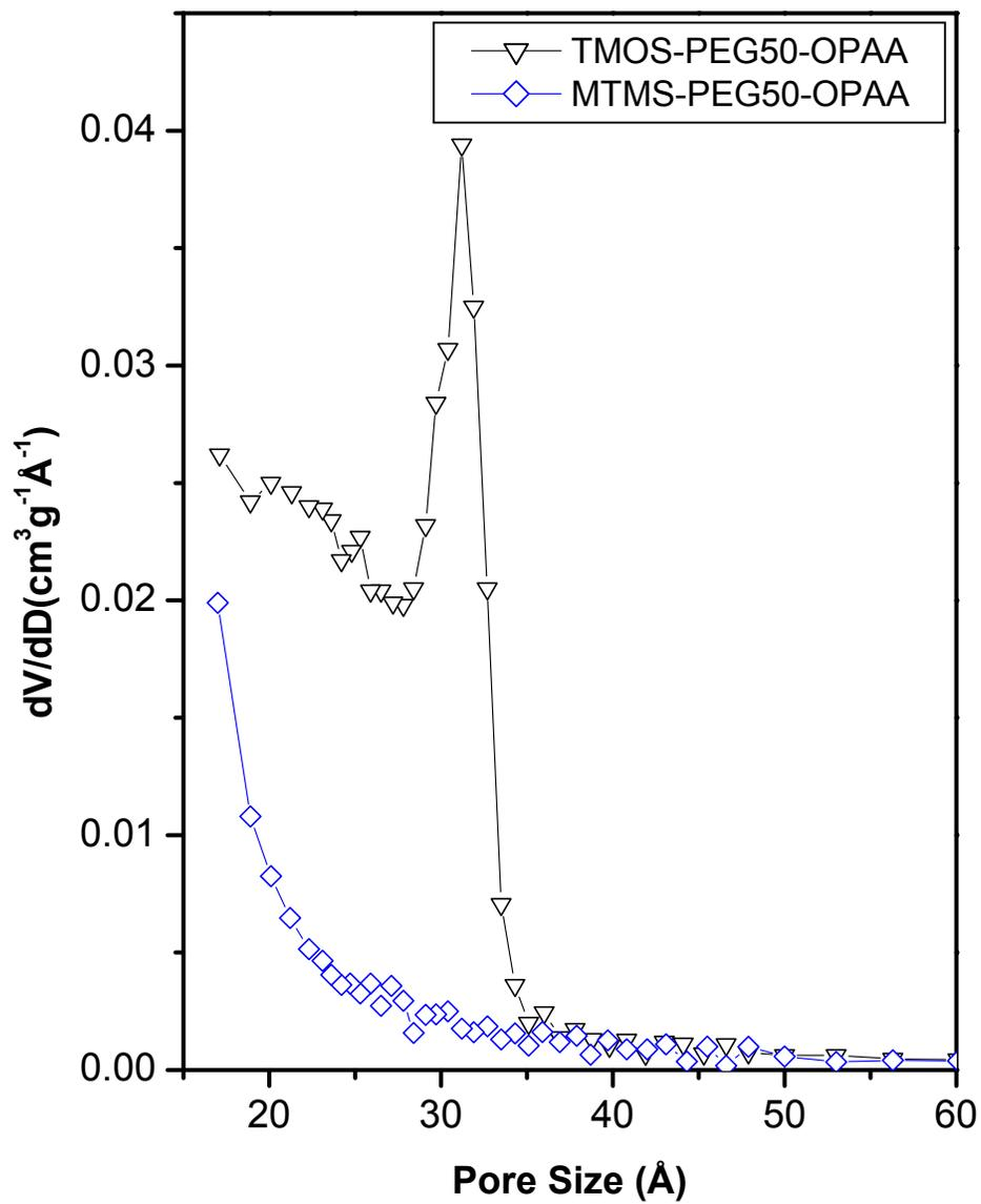
Figure 6. The BJH desorption pore size distributions from the N<sub>2</sub> desorption isotherms for the OPAA-containing hybrid sol-gel samples synthesized in the presence of 50 wt % PEG (MW 400).
