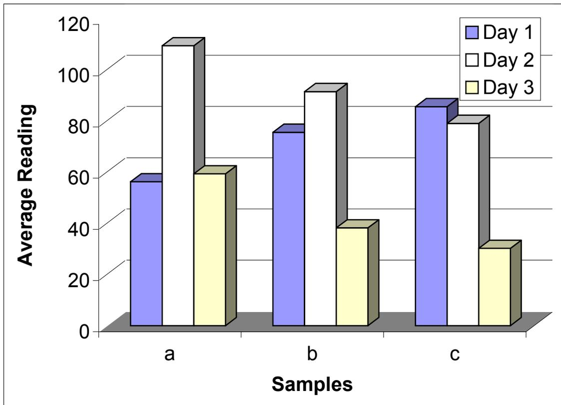
Figure 12. Stability of immobilized OPAA in methanol. (a) TMOS-F50-OPAA (b) TMOS-PEG50-OPAA (c) MTMS-PEG50-OPAA.
