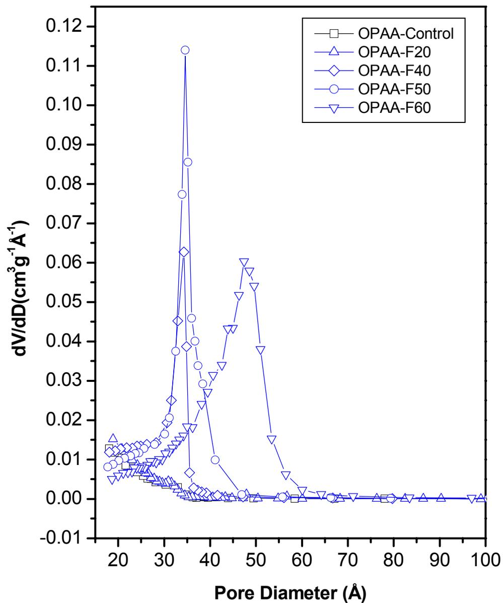
Figure 2 The BJH desorption pore size distributions from the N<sub>2</sub> desorption isotherms for the OPAA-containing hybrid sol-gel samples synthesized in the presence of 0-60 wt % D-fructose.
