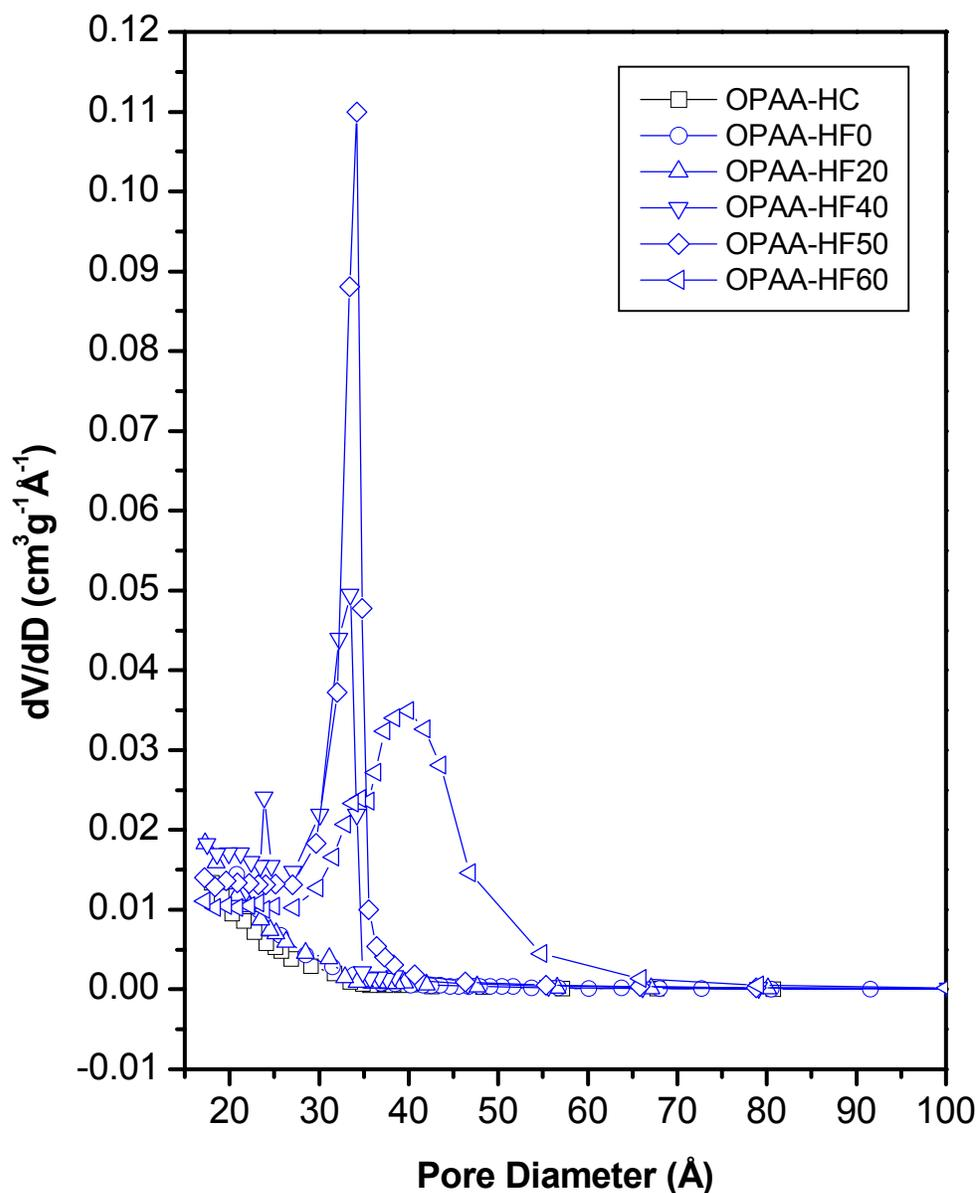
Figure 4. The BJH desorption pore size distributions from the N<sub>2</sub> desorption isotherms for the OPAA-containing hybrid sol-gel samples synthesized in the presence of 0-60 wt % D-fructose. The precursors composed of 75 mol% TMOS and 25 mol% MTMS.
