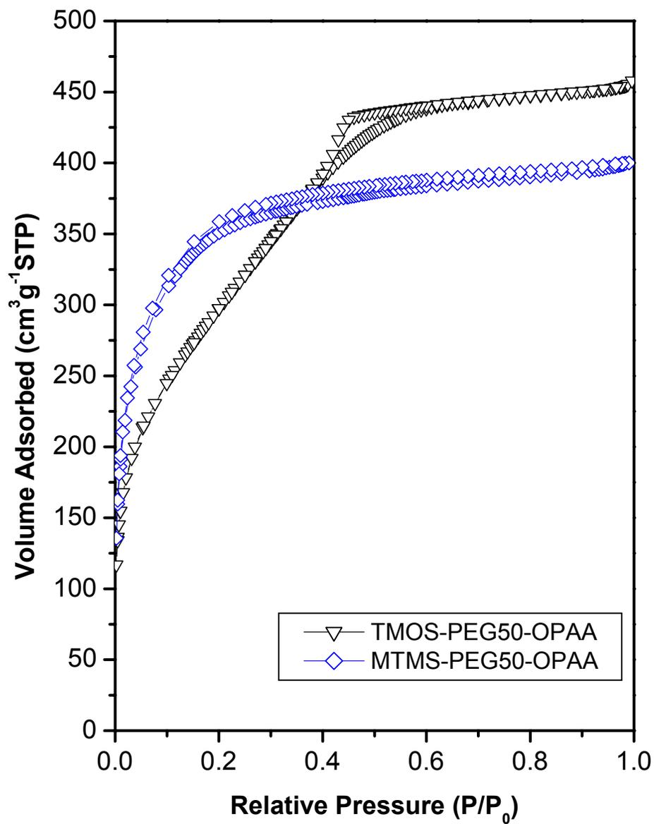
Figure 5. N<sub>2</sub> adsorption-desorption isotherms at -196 °C for the water-extracted OPAA-containing sol-gel matrices synthesized in the presence of 50 wt % PEG (MW 400).
