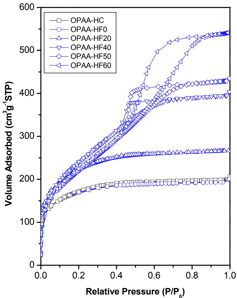
Figure 3. N<sub>2</sub> adsorption-desorption isotherms at -196 °C for the water-extracted OPAA-containing hybrid sol-gel matrices synthesized in the presence of 0-60 wt % D-fructose. Precursors is composed of 75 mol% TMOS and 25 mol% MTMS.
