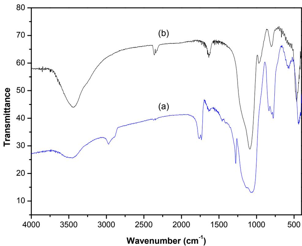
Figure 7. FT-IR of OPAA-containing samples synthesized from the hydrolysis of TMOS in the presence of 50 wt% fructose as template. (a) before water extraction (b) after water extraction.
