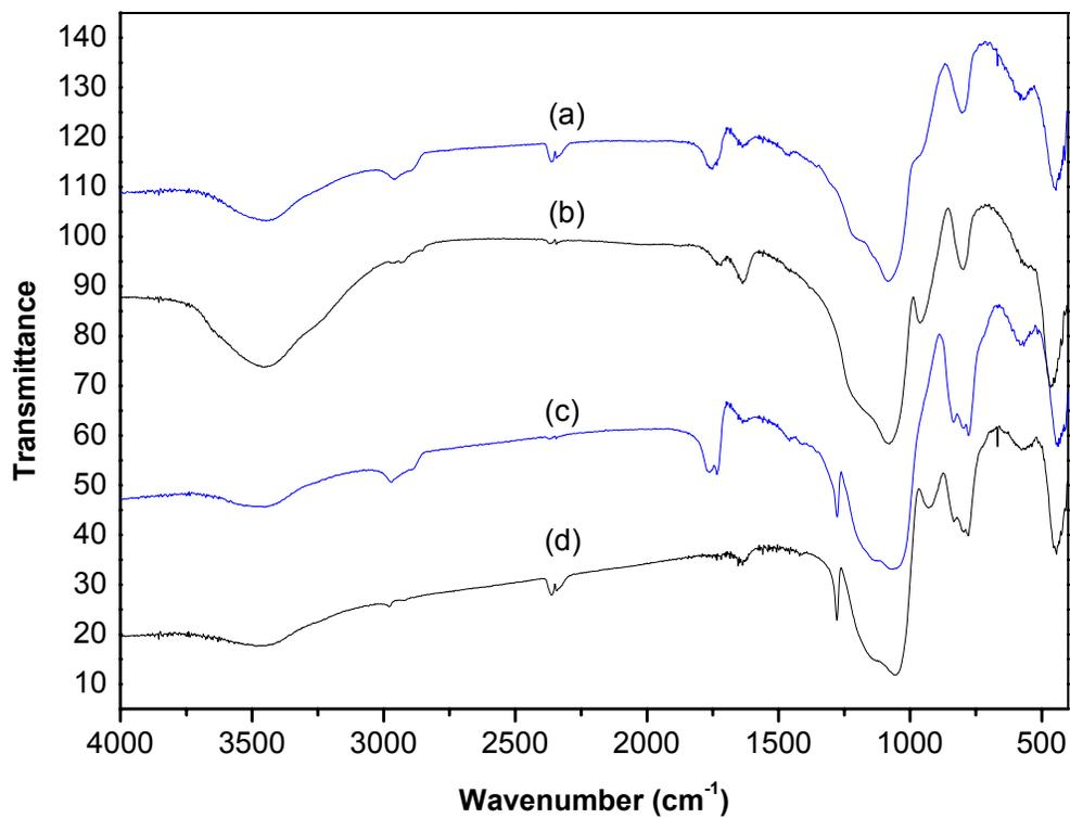
Figure 8. FT-IR of OPAA-containing samples synthesized from the hydrolysis of TMOS or TMOS/MTMS(1:1) in the presence of 50 wt% PEG as template. (a) TMOS, before water extraction (b) TMOS, after water extraction (c) TMOS/MTMS, before extraction (d) TMOS/MTMS, after extraction.
