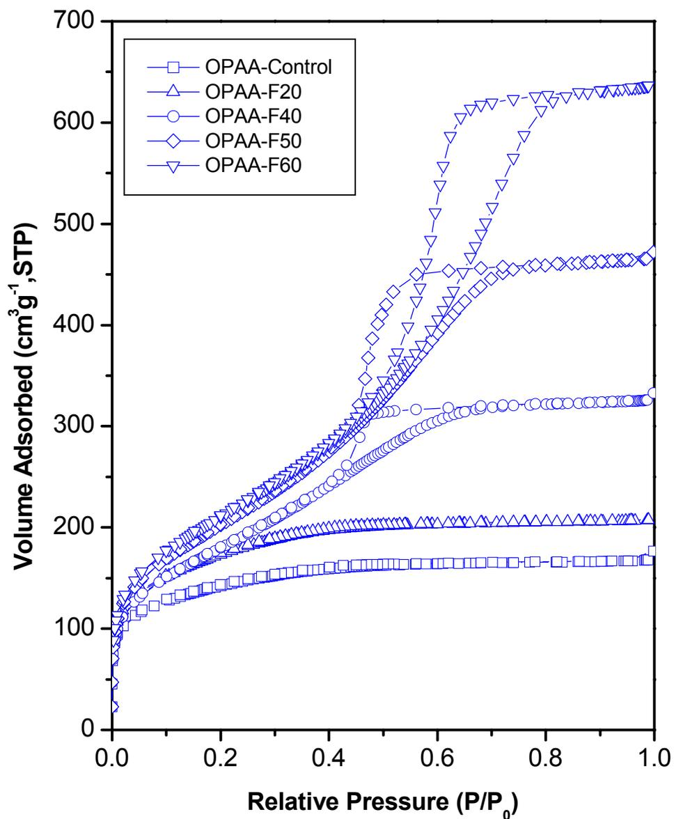
Figure 1. N<sub>2</sub> adsorption-desorption isotherms at -196 °C for the water-extracted OPAA-containing sol-gel matrices synthesized in the presence of 0-60 wt % D-fructose.
