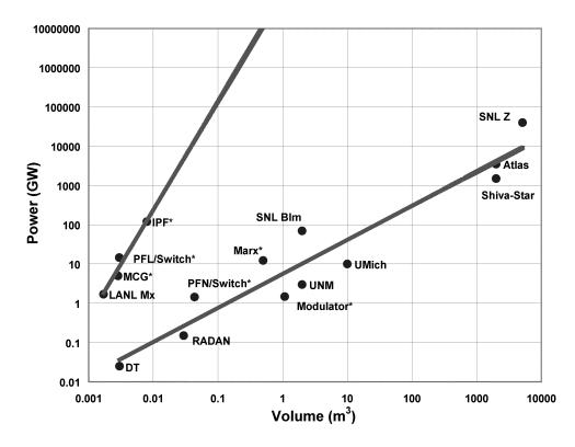
**Fig. 2.** The analogy of the mouse-to-elephant curve in pulsed power. The line with the faster rising slope comprises systems either driven by explosives or that use state-of-the-art high energy density components. The line with the lower slope represents more traditional pulsed power systems found in the laboratory. (Parameters for the sources denoted with an asterisk were obtained from [2].)
