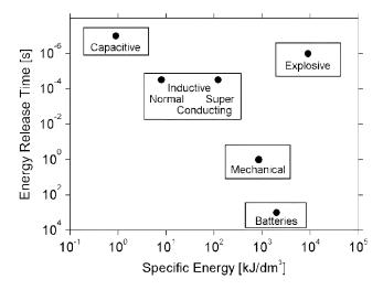
**Fig. 3.** Approximate specific energy and energy release time for diverse types of energy storage. (The explosive energy storage does not include the efficiency of transforming mechanical into electrical energy.)
