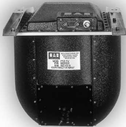
Pan-Tilt-Zoom Daylight Color TV BAI's electronically stabilized color TV sensor features an on-screen crosshair overlay. Encoders mounted on the gimbal's drive motors report sensor position via the payload's serial (RS-232) port.
