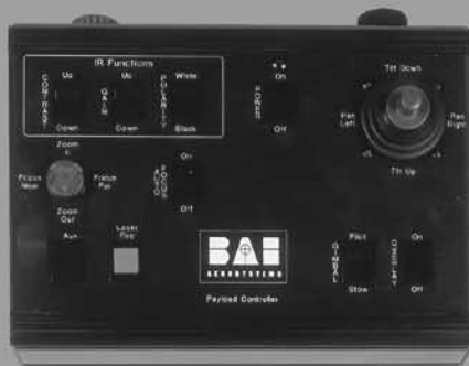
One Payload Controller is compatible with all three of the Dragon Drone's payloads.
