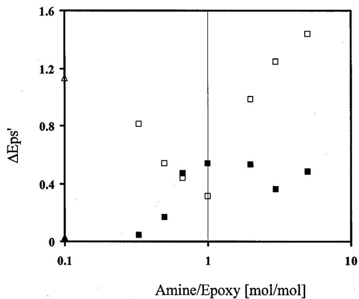
Figure 4.2.1.5 Dielectric relaxation strength of  $\beta$  and  $\gamma$  processes at different E:A ratios. Solid and open squares describe the  $\beta$  and the  $\gamma$  process of networks, respectively. Triangles (on the ordinate) describe  $\beta$  and  $\gamma$  processes in the neat DGEBA.
