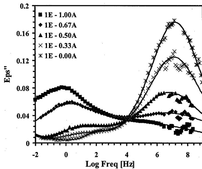
Figure 4.2.1.4 Dielectric loss in the frequency domain for a series of epoxy-rich DGEBA-DETA networks and neat DGEBA measured at  $-60^{\circ}\text{C}$ .
