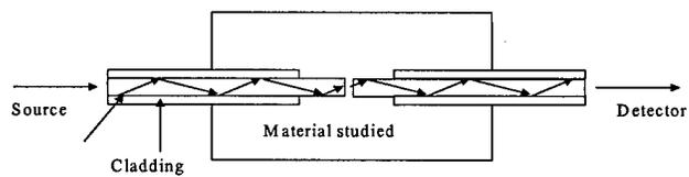
Figure 4.2.3.3 Mechanism of Tip-to-Tip method for NIR measurements.
