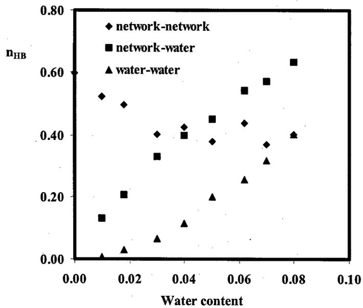
Figure 4.2.4.4 Number of HBs between network polar groups, between water and network polar groups, and between different water molecules as a function of water content.  $n_{HB}$  values are normalized per hydroxyl group of the polymer network.
