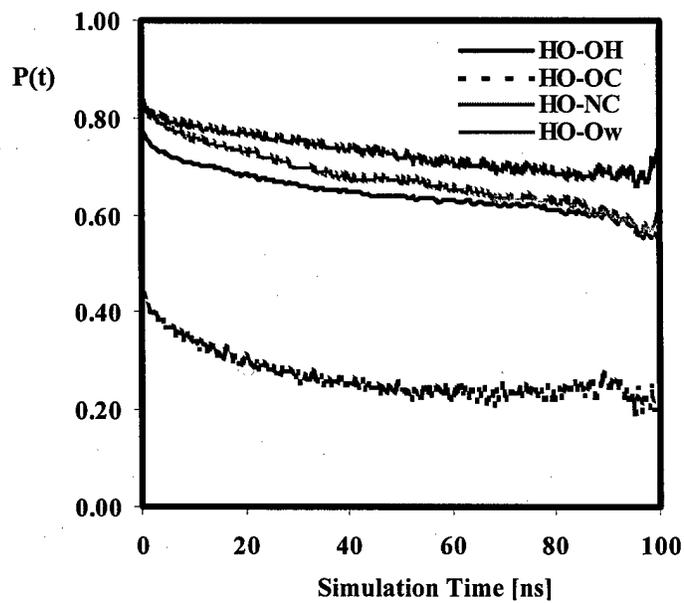
Figure 4.2.4.7 Correlation function,  $c(t)$ , for HBs of HO with different acceptors as a function of simulation time. Water content is 2% by weight.
