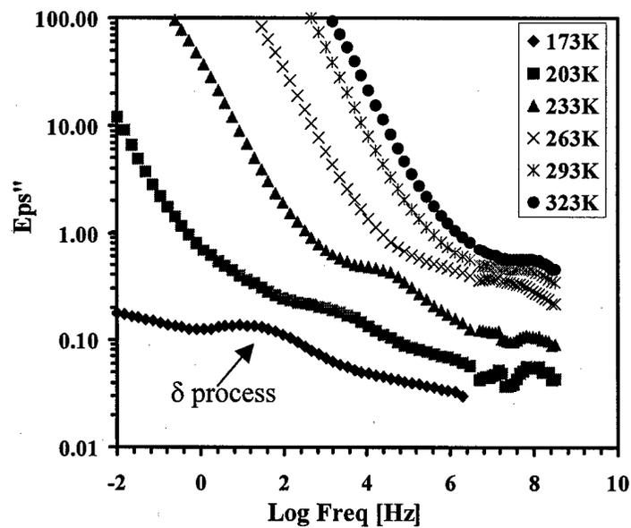
Figure 4.2.1.28 Dielectric spectra of DGEBA-DETA sample aged in 100°C water for 3517 hours with measuring temperature as a parameter..
