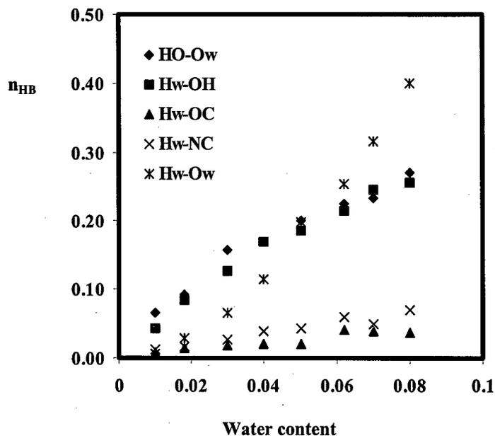
Figure 4.2.4.3 Number of HBs between water and polar groups of the polymer network, and between different water molecules as a function of water content,  $n_{HB}$  values are normalized per hydroxyl group of the polymer network.
