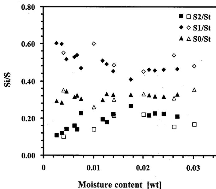
Figure 4.2.1.19 Relative ratio of the three forms of absorbed water ( $S_0$ ,  $S_1$  and  $S_2$ ) to the total water content ( $S_t$ ) as a function of moisture content. Solid symbols represent NIR results, open symbols the results from molecular simulations.
