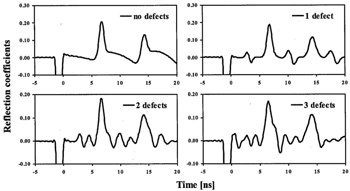
Figure 4.1.2.3 TDR responses of 150 mm water strip with 0, 1, 2, and 3 Teflon patches. The 1st, 2nd and 3rd patch were put at  $\frac{1}{2}$ ,  $\frac{3}{4}$ , and  $\frac{1}{4}$  of the water strip length from the connector.
