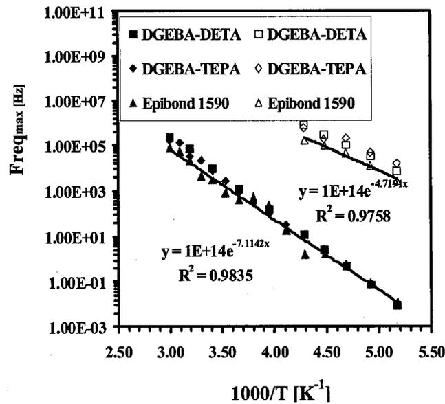
Figure 4.2.1.9 Frequency at maximum loss as a function of reciprocal temperature for DGEBA-DETA, DGEBA-TEPA and Epibond 1590 system. Solid and open symbols describe the  $\beta$  and the  $\gamma$  process, respectively.
