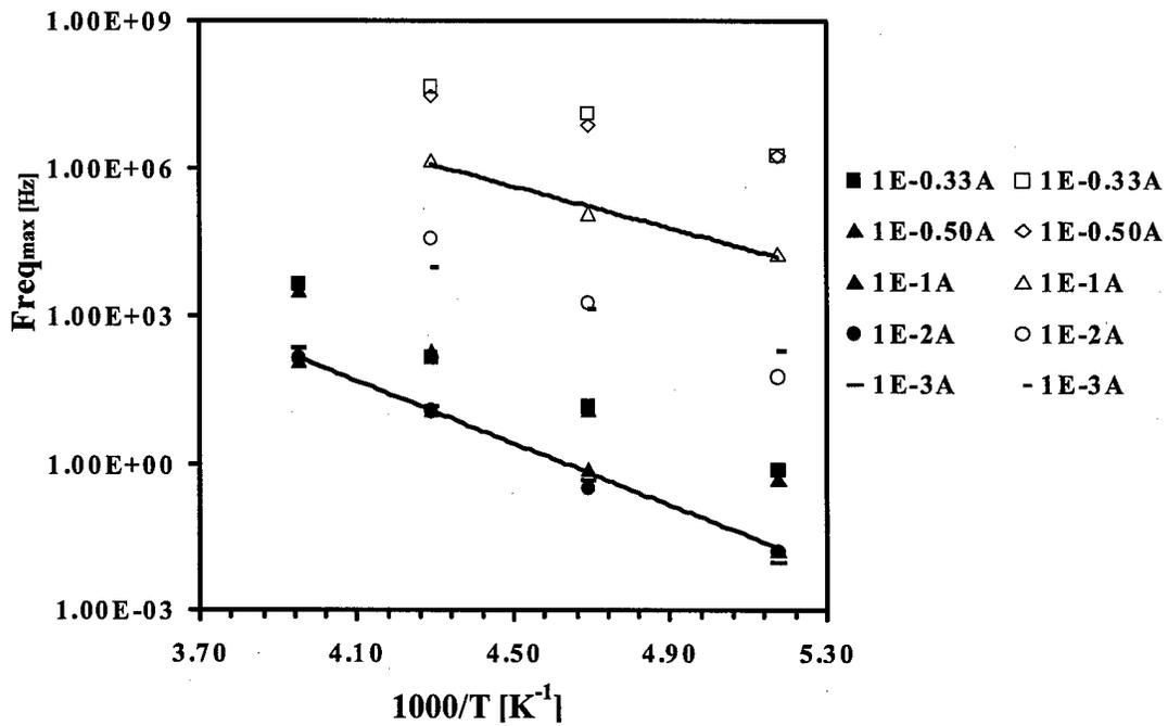
Figure 4.2.1.6 Frequency at maximum loss as a function of reciprocal temperature for a series of stoichiometric and off-stoichiometric networks. Solid and open symbols describe the  $\beta$  and the  $\gamma$  process, respectively.
