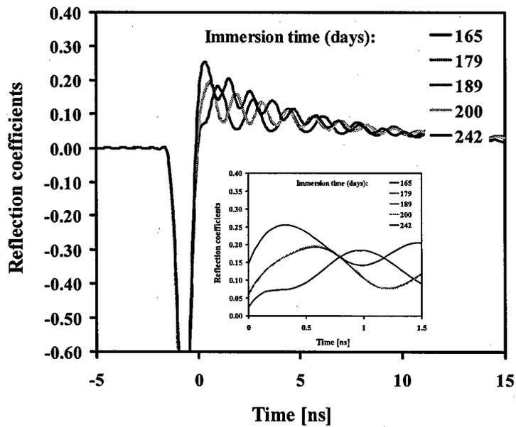
Figure 4.2.2.2 TDR traces of “imperfect” joint for aging time shorter (upper) and longer (lower) than 165 days.
