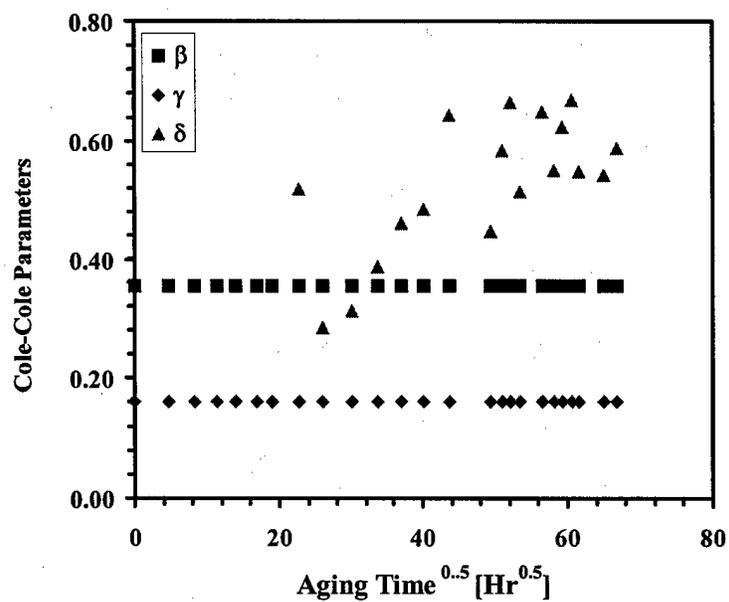
Figure 4.2.1.29 Cole-Cole parameters of  $\beta$ ,  $\gamma$  and  $\delta$  processes of DGEBA-DETA system as a function of water content (upper figure) and aging time (lower figure).
