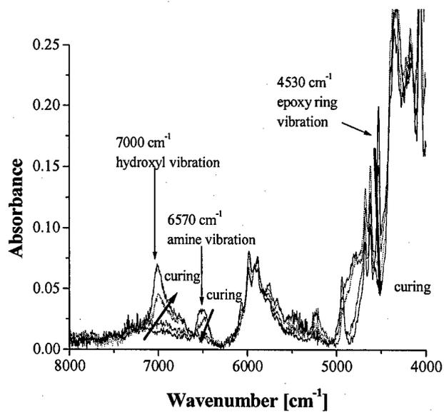
Figure 4.2.3.4 Tip-to-Tip NIR spectra of DGEBA-DETA mixture during cure. The curing procedure consists of three steps: 1) room temperature for 180 min, 2) 60°C for 90min, and 3) 130°C for 60min. In the direction of bold arrows, the spectra were scanned before cure, after the 1st, 2nd and 3rd step of cure, respectively.
