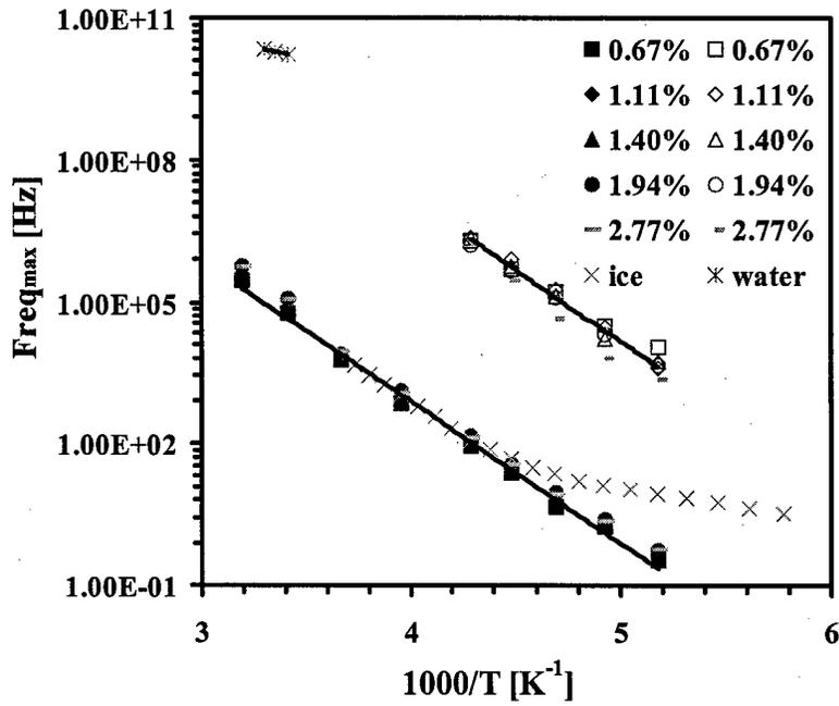
Figure 4.2.1.15 Frequency at maximum loss as a function of reciprocal temperature for  $\beta_m$  (solid symbols) and  $\gamma_m$  (open symbols) relaxations, with moisture content as a parameter. Also shown are the frequency at maximum loss data for ice (X) and liquid water (\*).
