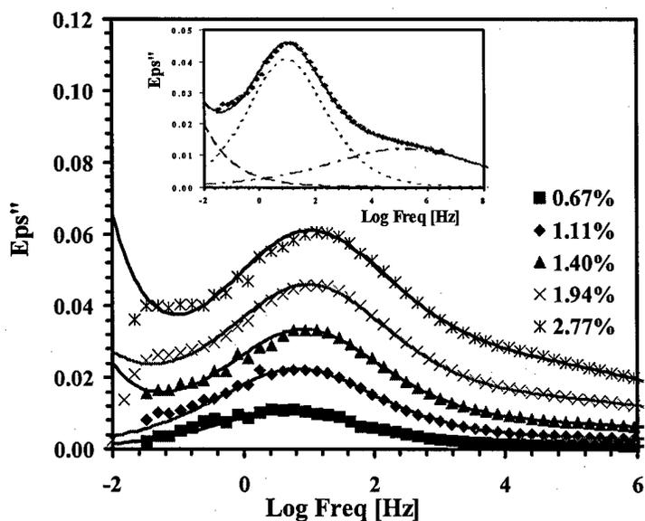
Figure 4.2.1.14 Difference dielectric spectra of 1E:1A DGEBA-DETA network in the frequency domain with moisture content as a parameter, measured at  $-60^{\circ}\text{C}$ . The inset shows a deconvoluted difference spectrum of 1E:1A DGEBA-DETA network with the aid of two Cole-Cole functions and a low-frequency dc conductivity dependence (with 1.94% moisture, measured at  $-60^{\circ}\text{C}$ ).
