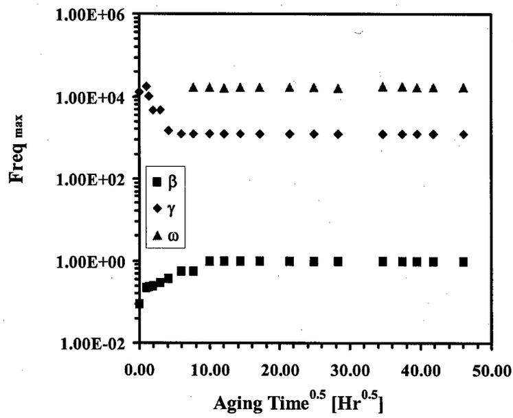
Figure 4.2.1.41 Frequency at maximum loss of β, γ and ω processes in Epibond 1590 as a function of water content (upper figure) and aging time (lower figure).
