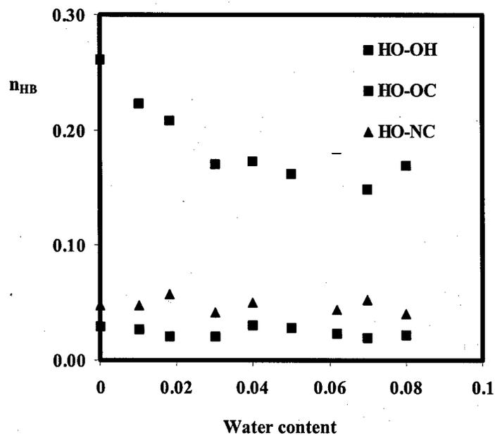
Figure 4.2.4.2 Number of HBs between polar groups of the polymer network as a function of water content.  $n_{HB}$  represents an average per hydroxyl hydrogen of the polymer network.
