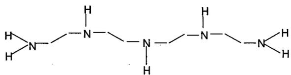
Figure 4.2.1.1 Chemical structure of tetraethylene pentamine (TEPA).
