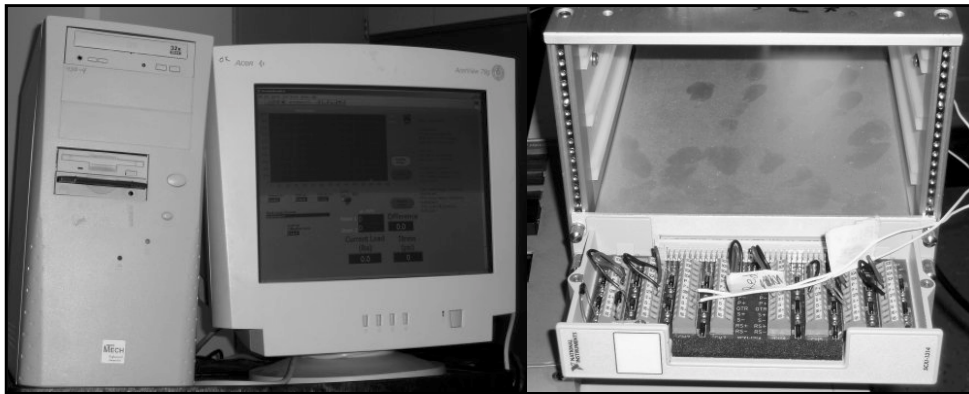
Figure 5.2.22 Data Acquisition Computer and 8 Channel Terminal Block
