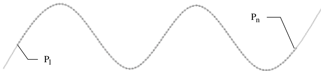
Figure 2.6.4 Cross Section of Figure 2.6.3 Surface Shows Defining Points
