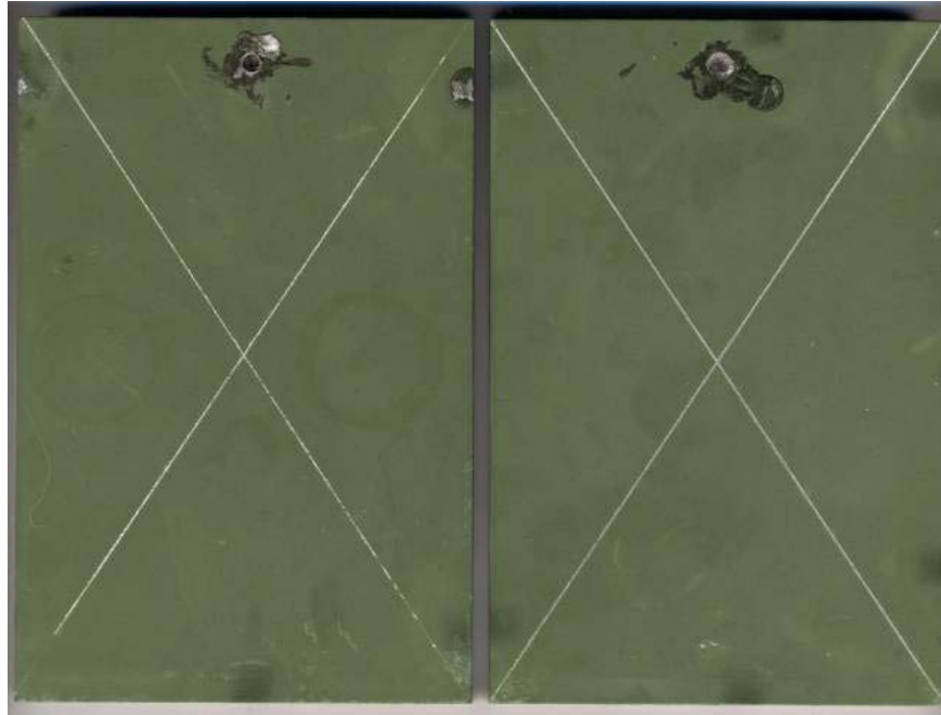
Figure 8. Grit-blasted 2519 after 48 months of exposure.
