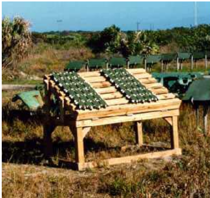
Figure 1. Exposure racks at Cape Canaveral.
