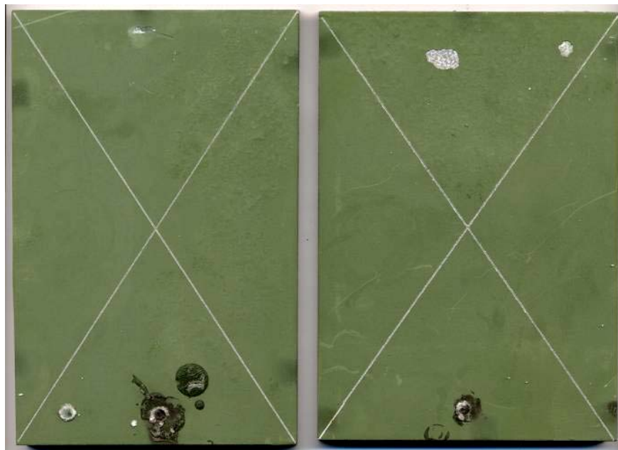
Figure 9. Grit-blasted 7039 after 48 months of exposure.
