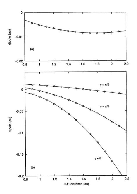
Figure 7. Dependence on R of (a) the rovibrationally averaged Ar-H<sub>2</sub> dipole moment  $\langle M \rangle_{00}$  and (b) the Ar-H<sub>2</sub> Q<sub>1</sub>(0) transition dipole moment  $\langle M \rangle_{01}$ . The solid lines are cubic spline fits to the data. Note the change from linear to logarithmic scale in each plot at  $\langle M \rangle = -2 \times 10^{-5}$  au.
