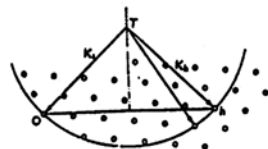
FIG. 5. Geometrical theory of space lattice diffraction in Fourier space.
