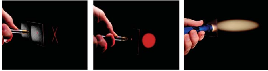
Figure 7 Typical diffuser illumination schemes described by Eq. (22) for various diffuser FWHM angular values.
