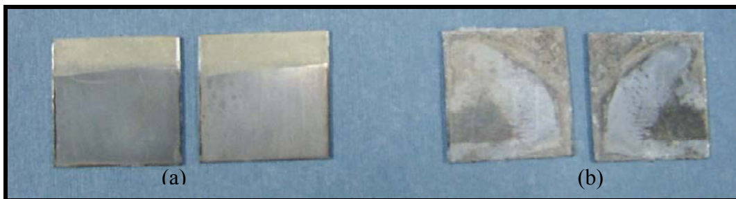
FIGURE 5. Aluminum AA7075 1x1 inch plates after 48h, 0.15 M NaCl corrosion test by capillary effects in the interior of the artificial crevice (a) Polystyrene coated, (b) Bare aluminum.
