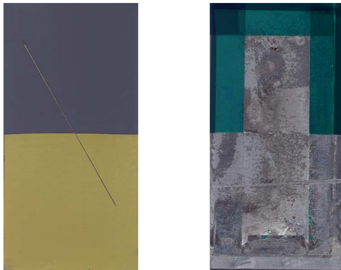
FIGURE 5. AC7-6: Epoxy-zirconate sol-gel pretreatment, 23377 chromated primer, 3M appliqué (non-perforated).
