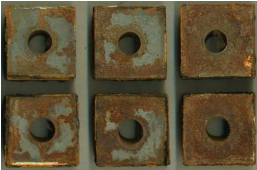
FIGURE 7b. Macrophotos of Ti-steel Interfaces after Phase II Salt Fog Exposure
