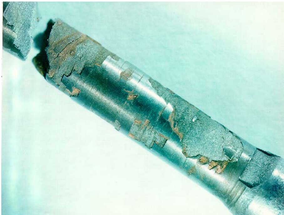
FIGURE 4(b) Flaking of HVOF Coating during SCC Test
