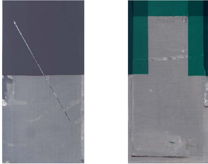
FIGURE 4. AC8-17: SNAP sol-gel pretreatment, 3M appliqué (non-perforated).
