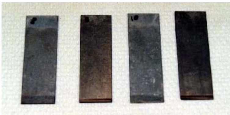
FIGURE 3. ISAM coated aluminum 2024 samples after 168 hour salt fog test showing corrosion inhibition. "Speckle" in the photo is not corrosion, but reflectivity properties of the aluminum samples under the light of the photoflash.
