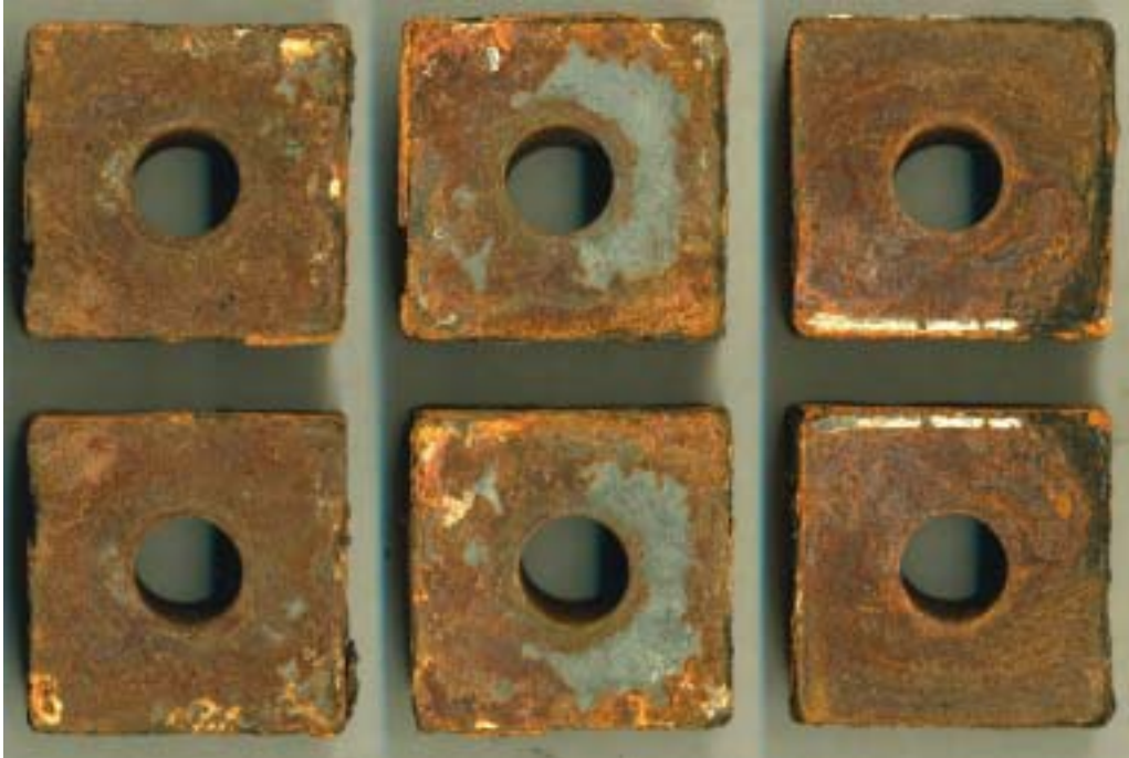
FIGURE 10a. Macrophotos of Fe-Fe Interfaces after Phase II Salt Fog Exposure
