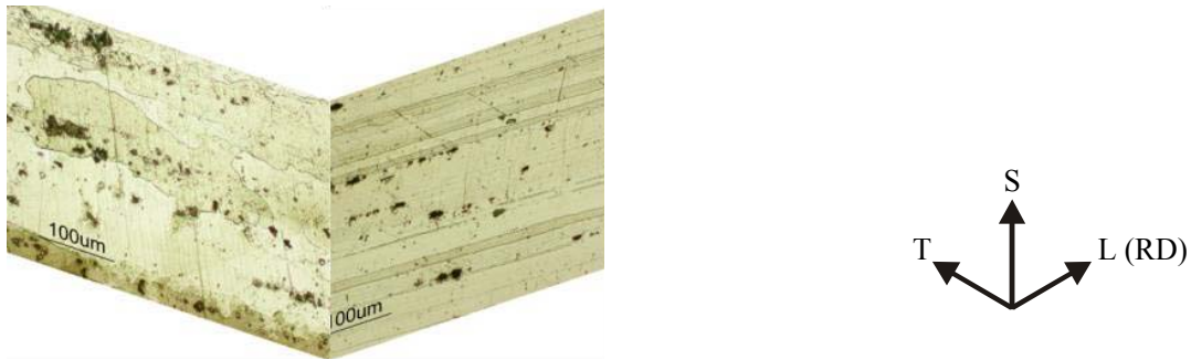
FIGURE 1. Microstructure of 1 in. thick plate of AA 7075-T651 used in this study. RD = rolling direction.
