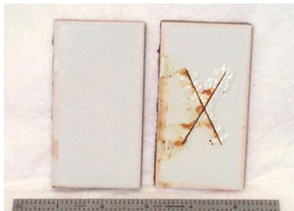
FIGURE 4: Physical appearance of carbon steel panels after testing.
