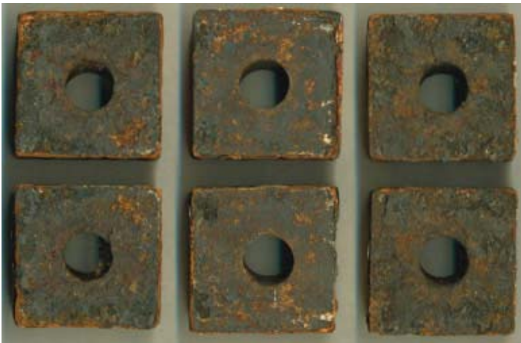
FIGURE 10b. Macrophotos of Fe-Fe Interfaces after Phase II Cyclic Corrosion Exposure
