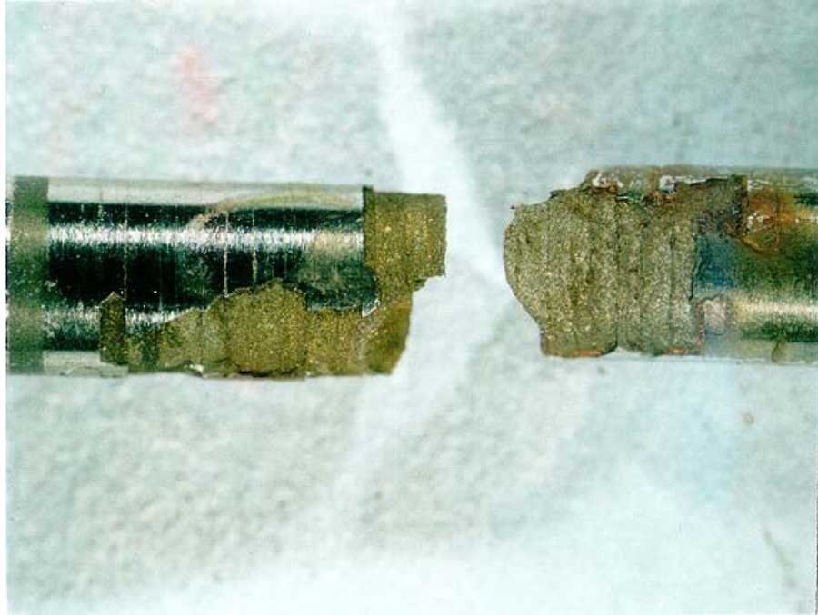
FIGURE 4(a) Flaking of Cr Plating during SCC Test
