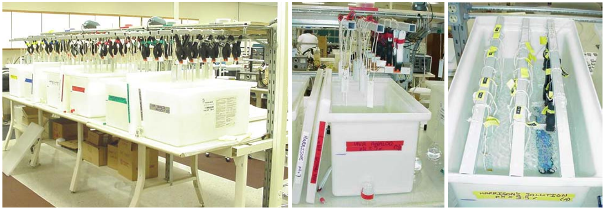
FIGURE 1: Test setup showing tanks and panels suspended from racks (left), one tank with panels suspended from racks above tank (middle) and in the tank (right).
