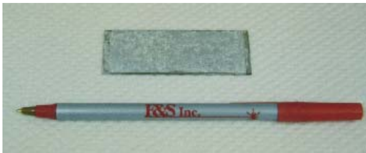
FIGURE 2. LUNA uncoated aluminum 2024 coupon after salt fog test, showing severe corrosion.
