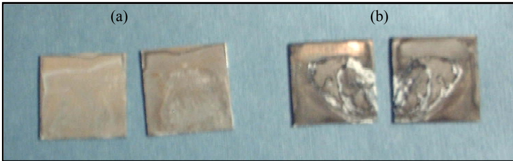
FIGURE 6. Aluminum AA7075 1x1 inch plates after 168h, 3.5 w% NaCl corrosion test by capillary effects in the interior of the artificial crevice, (a) Polystyrene coated, (b) Bare aluminum.
