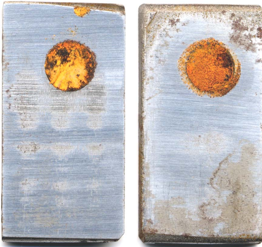
FIGURE 6. Corrosion Products on AISI 4130 after 14 Days Galvanic Cell Test ( left sample #4 exposed to 0.5N NaCl; right sample #2 exposed to 0.005N NaCl).
