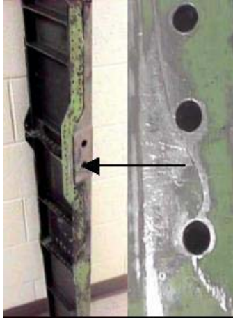
FIGURE 1: Close up of SH-60 transmission beam fatigue crack
