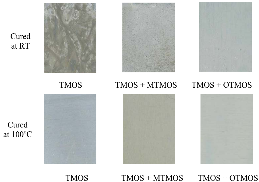
FIGURE 2: Effect of organosilanes on alternate immersion of coated aluminum panels in 3.5% NaCl solution. MTMOS and OTMOS were added into SNAP formulations. Visual photographs taken after three weeks.
