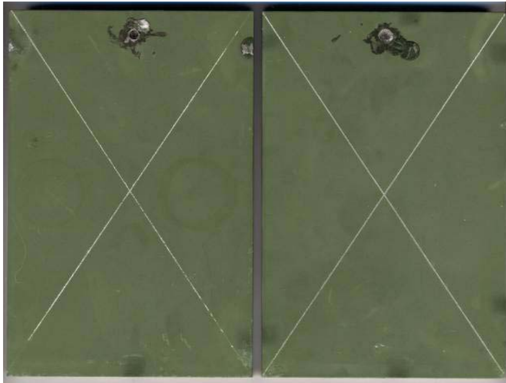
FIGURE 17: Grit Blasted 2519 after 48 months exposure
