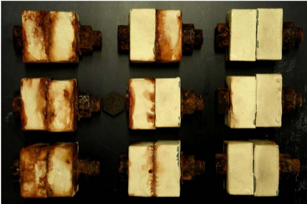
FIGURE 8. Assembled Armor Mockup Couples after Phase II GM 9540P Testing Exposure
