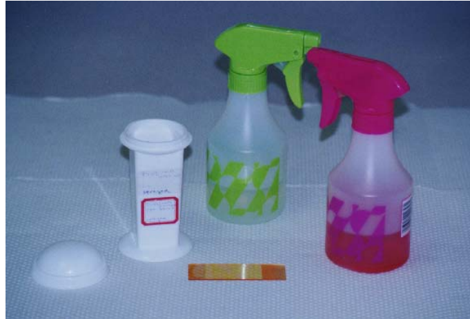
FIGURE 8. Spray Coating ISAM Film Fabrication Apparatus and Sample Film.
