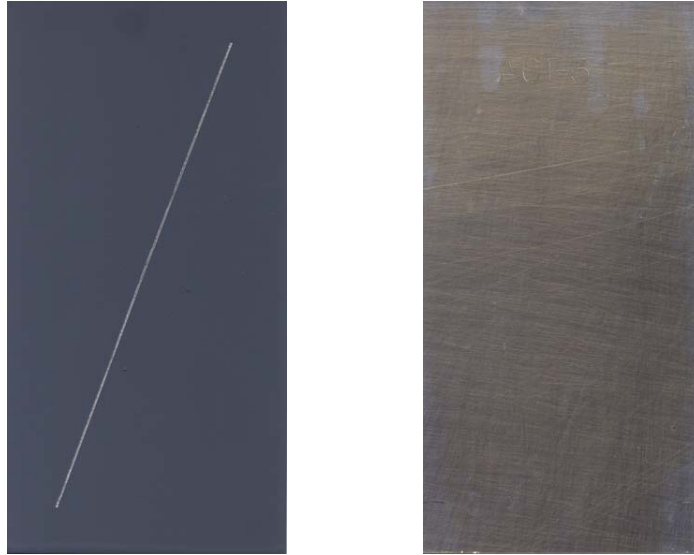
FIGURE 1. AC1-3 (control): Alumigold chromate conversion coat, 23377 chromated primer, 85285 topcoat.
