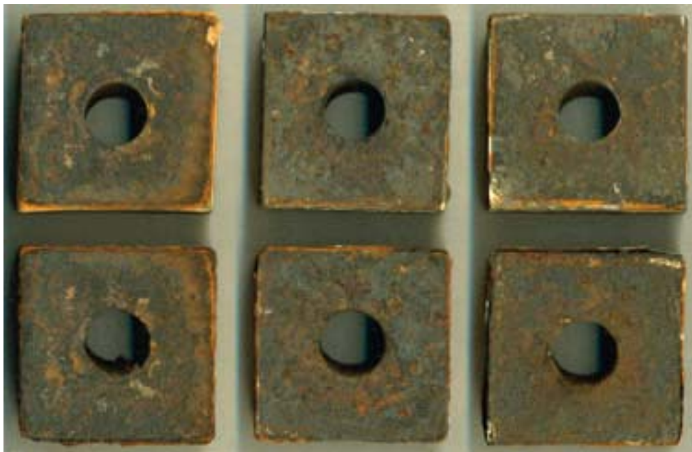
FIGURE 9b. Macrophotos of Ti-steel Interfaces after Phase II Cyclic Corrosion Exposure
