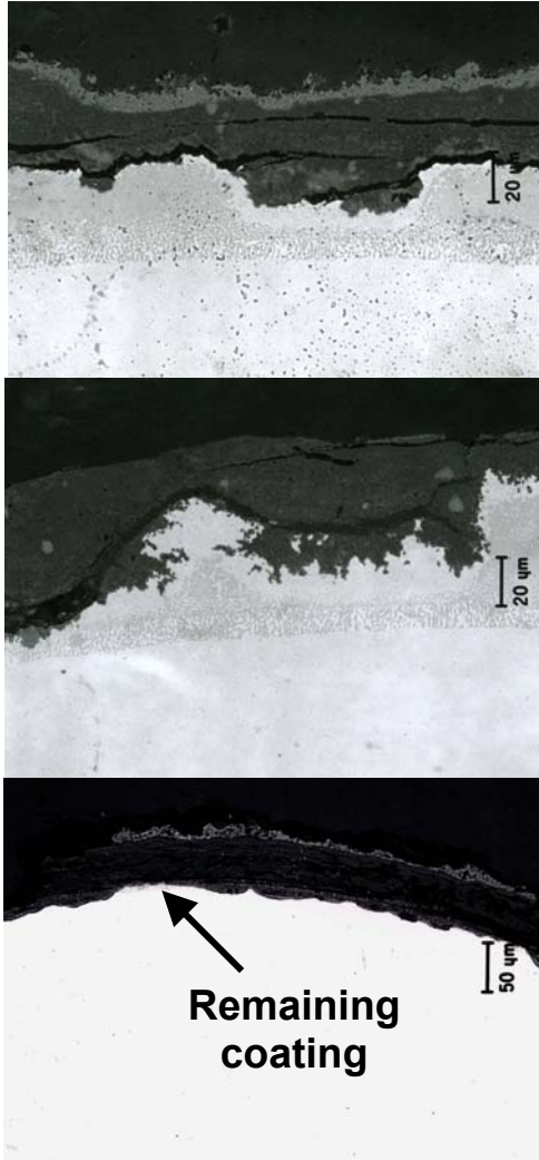
FIGURE 3. Alloy 738/Coating A after 1000-hr LVBR exposure at 1300 °F (704 °C) burning different fuels. The typical coating losses increased as the carbon residue content in the fuel increased. Coating degradation caused by Type II hot corrosion. Performance of Alloy 792/Coating A is similar.
