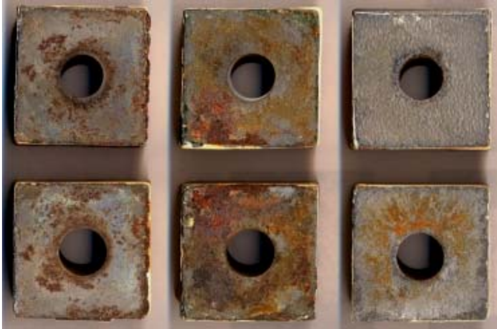
FIGURE 9a. Macrophotos of Ti-steel Interfaces after Phase I Cyclic Corrosion Exposure
