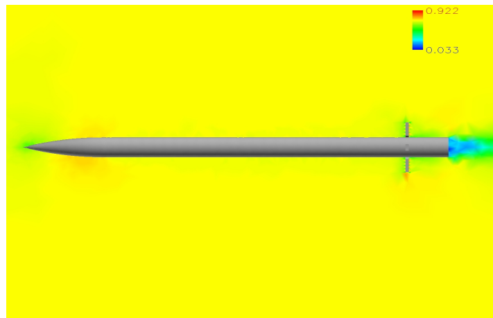
Figure 42: Numerical Mach Contours M=0.7 AOA=-5 deg
