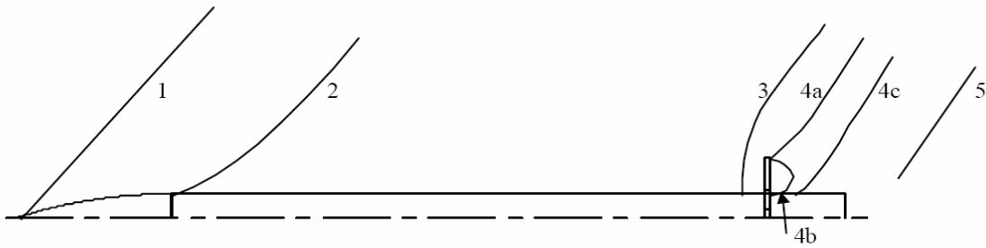
Figure 11: Flow around Missile with Mach Number Greater than 1 (13)
