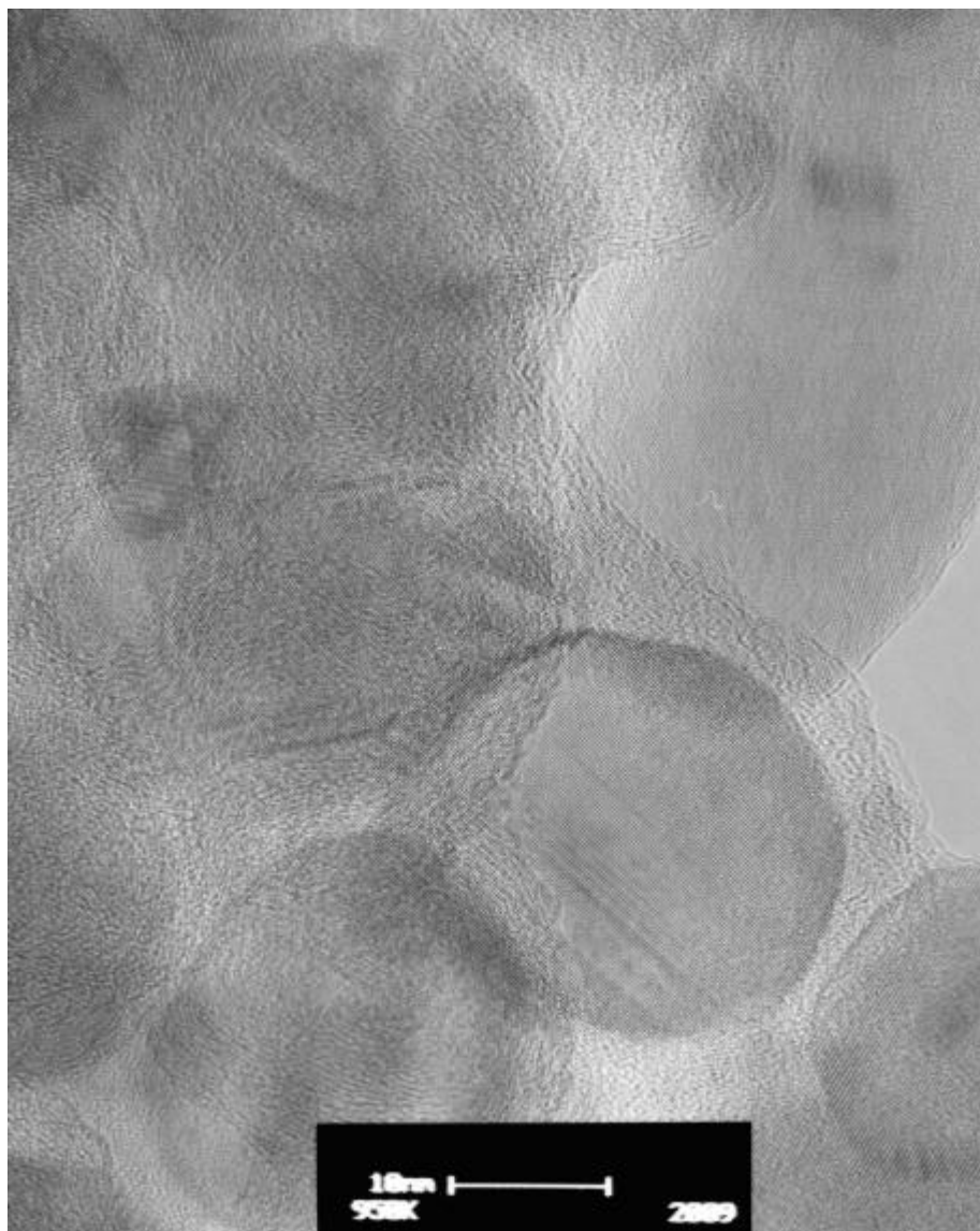
Chromium coating produced by magnetron sputtering ( t=400\text{nm} )
