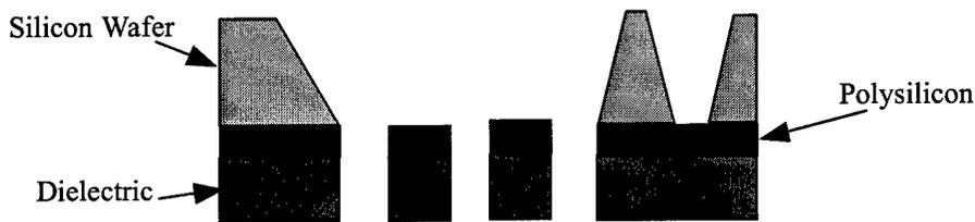
**Figure 17 - MEMS Gate Structure**
