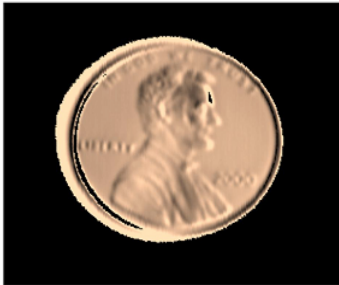
Figure 33. Eddy current map of a US penny obtained at 100 kHz using a commercial GMR sensor.
