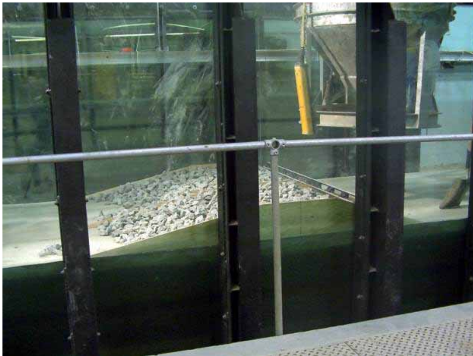
Figure A12. Construction of spur as seen through viewing windows at test section
