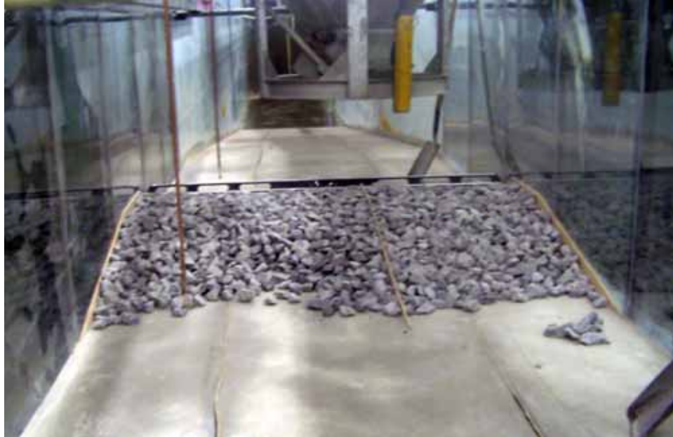
Figure A11. Construction of spur showing templates
