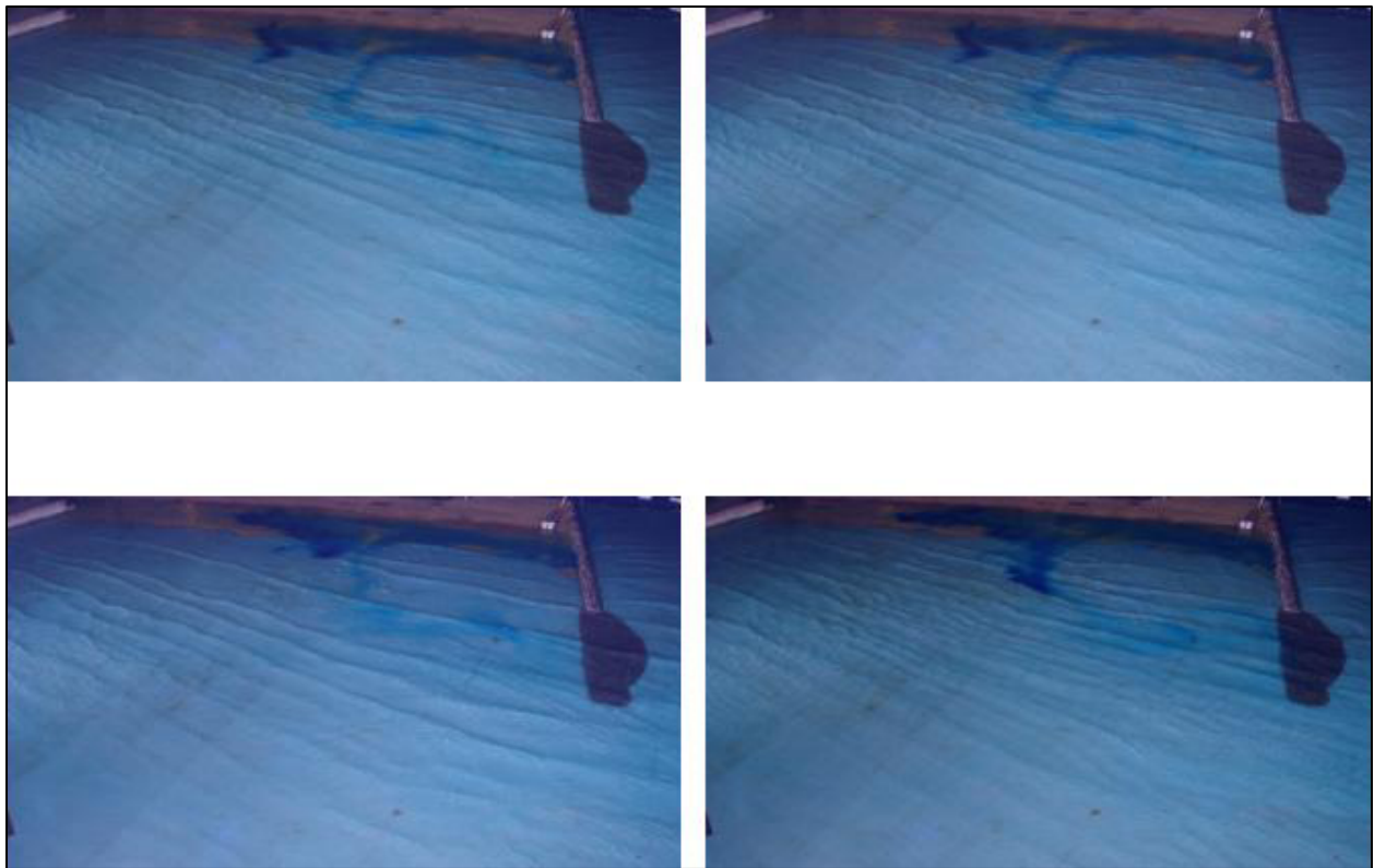
Figure B22. Dye study of 3-m, 13-sec waves from west-northwest at mhw, Alt 1
