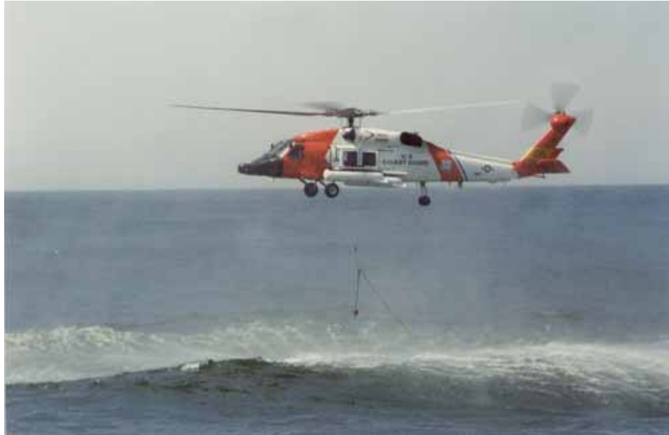
Figure D7. HH-60J helicopter (USCG Air Station Astoria) retrieving buoyant line and trailing float from surface with a grapnel at sta OS 5 (30 May 2001)
