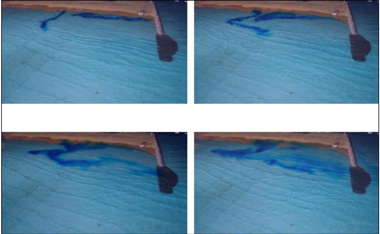
Figure B17. Dye study of 5-m, 13-sec waves from west-northwest at mllw, Alt 1
