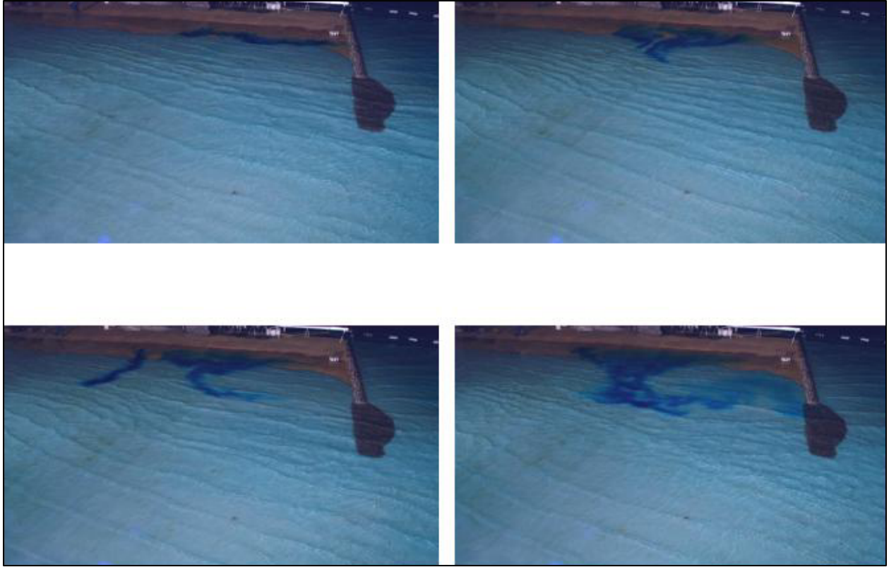
Figure B20. Dye study of 5-m, 13-sec waves from west-northwest at mtl, Alt 1, with full flood current
