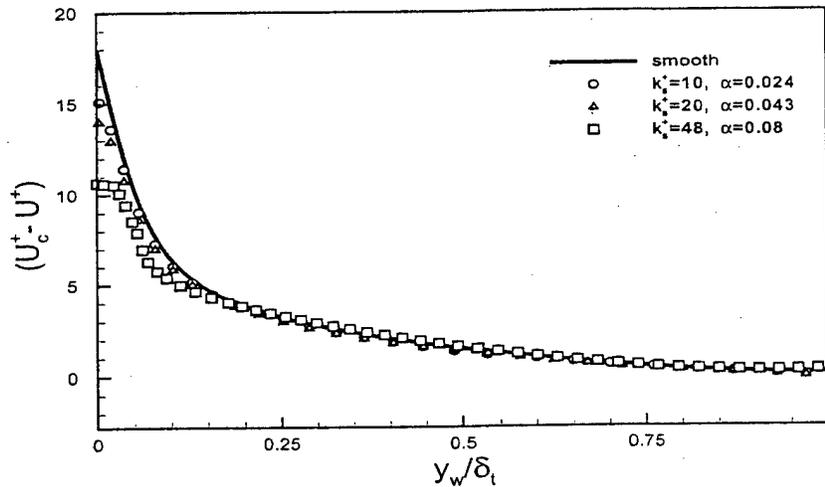
Figure 3: Mean velocity defect normalized by local  $u_\tau$ . The wall-normal distance is normalized by  $\delta_t$  (defined as the length from the wall to the  $y$ -location corresponding to the minimum rms velocity fluctuations from Fig. 4(a)), which is the effective boundary layer thickness.
