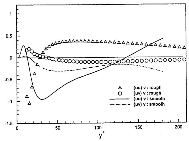
Figure 10: Reynolds stress transport terms,  $\overline{u^2v}$  and  $\overline{uv^2}$  (transport terms in  $\overline{u^2}$ - and  $\overline{uv^2}$ -budget respectively).
