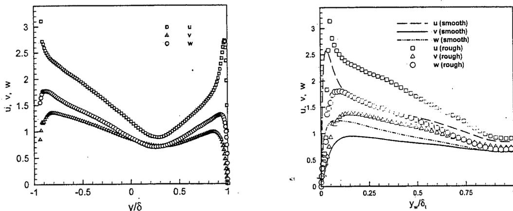
Figure 4: (a) Turbulent intensity of velocity components normalized by  $u_\tau$  at the smooth wall. The wall-normal distance is normalized by the channel half-height. (b) The wall-normal distance is normalized by  $\delta_t$ .
