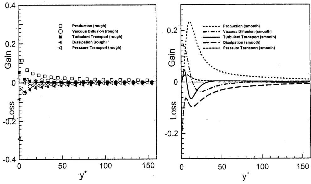
Figure 9: Terms in the turbulent kinetic energy budget normalized by local  $u_\tau$  and plotted in  $y^+$ .
