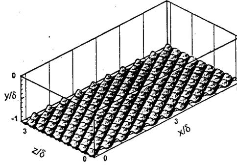
Figure 1: The roughness surface used in the simulations for  $h^+ = 21.6$ . The channel is shown from the lower-wall ( $y=-1$ ) to the center of the channel ( $y=0$ ). The virtual no-slip roughness surface is at  $\sigma = -0.96$ .
