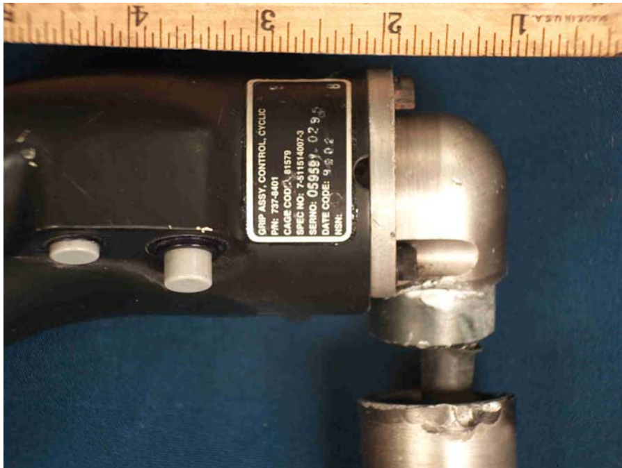
Figure 2. Enlargement of the fracture area on the pilot stick.
