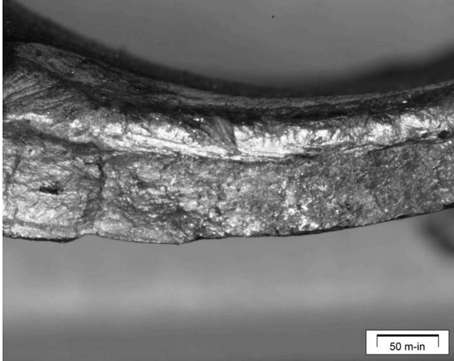
Figure 8. Lack of penetration on the tube side at location G on the drawing.
