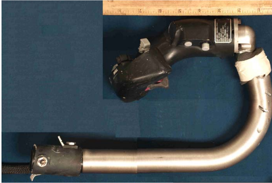
Figure 1. The fractured AH-64D pilot cyclic stick as received by ARL.
