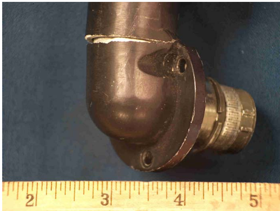
Figure 5. Detail of the copilot stick crack at the elbow to tube weld.
