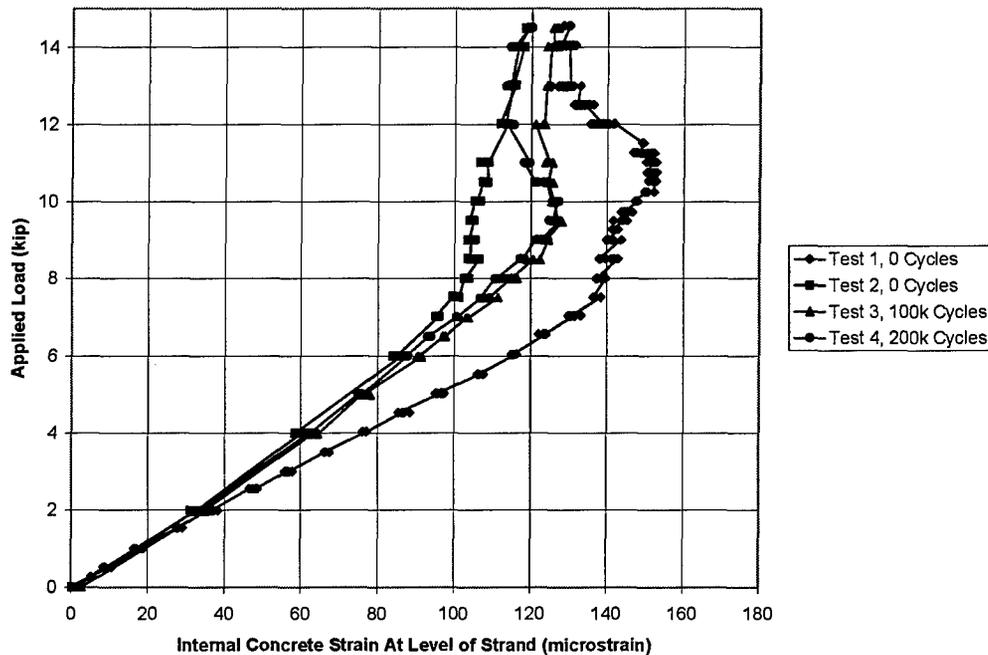
**Figure 4-24 Variation of Embedded Concrete Strain During Fatigue Tests—
