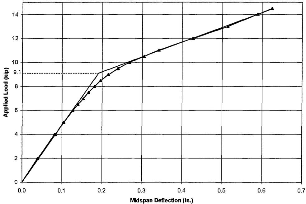
**Figure 4-19 Estimated Decompression Load Using Midspan Deflection—Beam 5**
