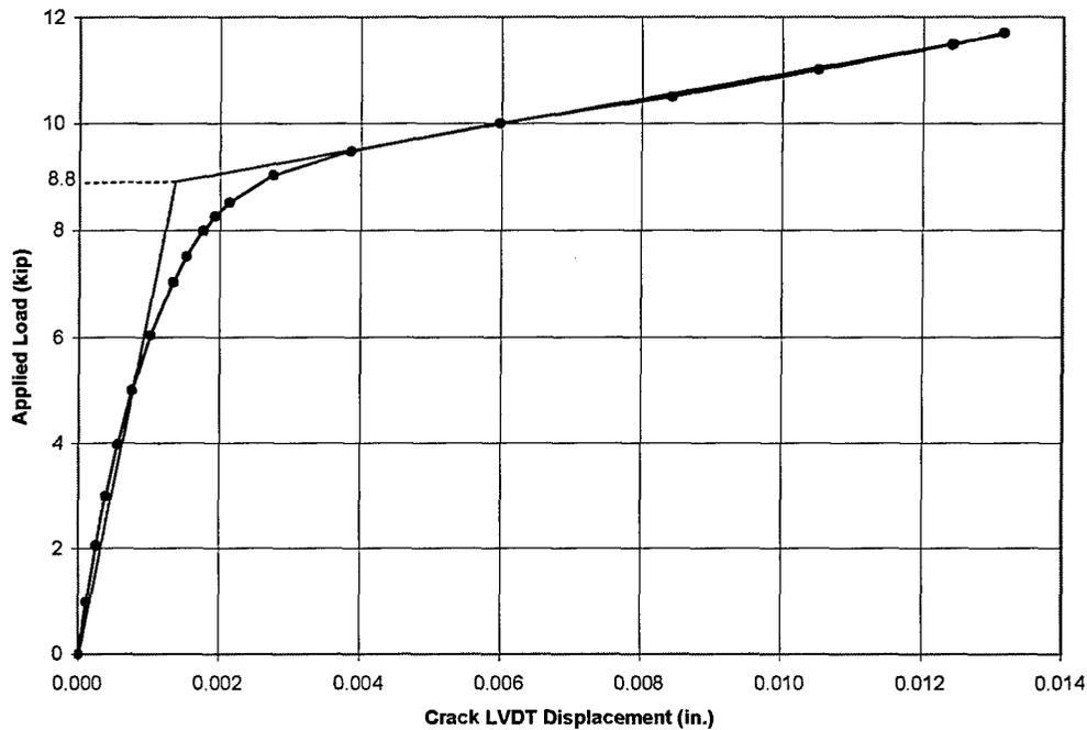
*Figure 4-54 Estimated Decompression Load Using Crack LVDT Displacement—Beam 2*
