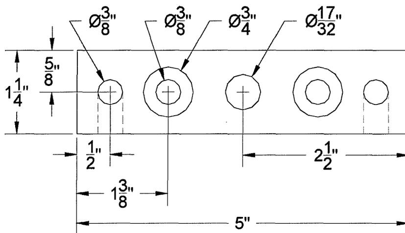
*Figure C-7 Top View of Bottom Aluminum Block*
