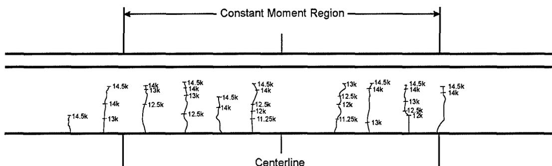
*Figure 4-17 Crack Pattern Following Initial Static Test—Beam 5*
