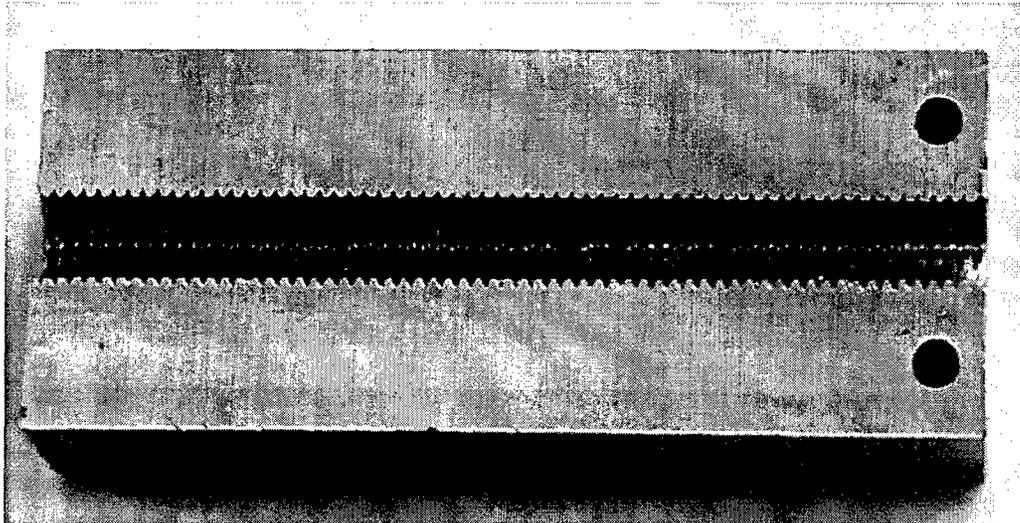
*Figure B-7 Interior Face of an Unused Threaded Grip*
