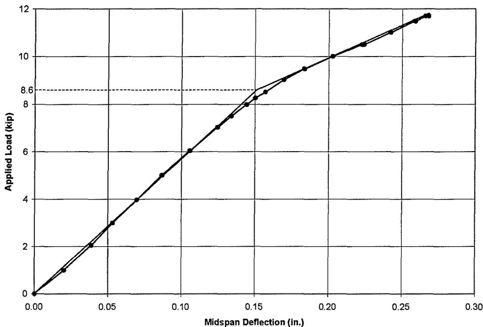
**Figure 4-53 Estimated Decompression Load Using Midspan Deflection—Beam 2**
