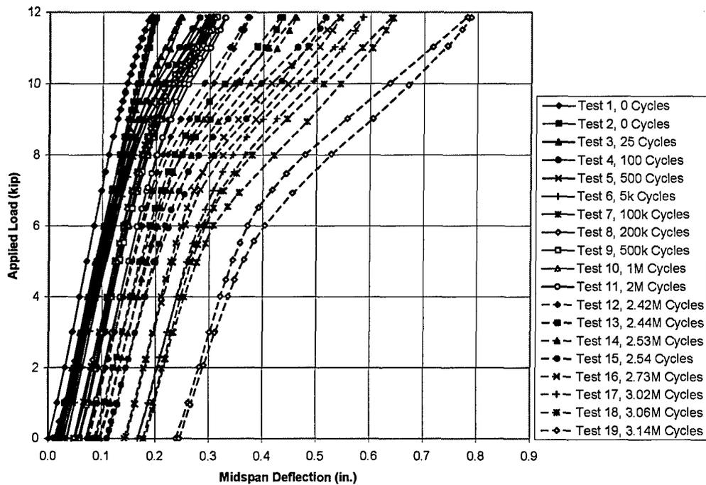
**Figure 4-39 Variation of Midspan Displacement, Including Permanent Offset—Beam 3**
