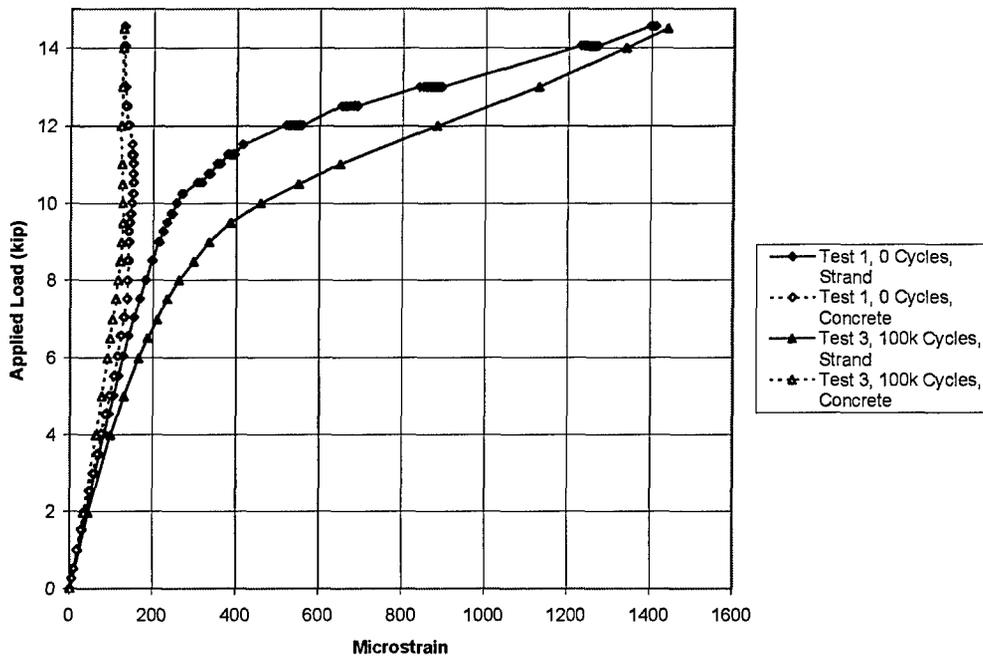
**Figure 4-25 Comparison of Strand Strain and Concrete Strain—Beam 5**
