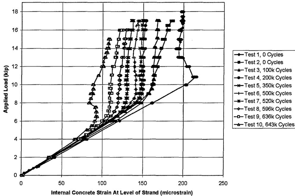
**Figure 4-7 Variation of Embedded Concrete Strain During Fatigue Tests—
