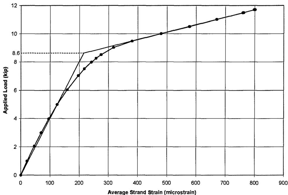
*Figure 4-52 Estimated Decompression Load Using Average Strand Strain—
