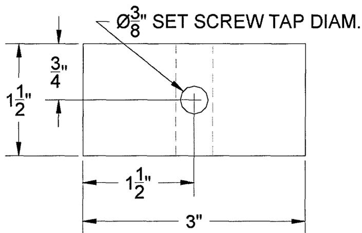
*Figure C-6 Front View of Middle Aluminum Block*
