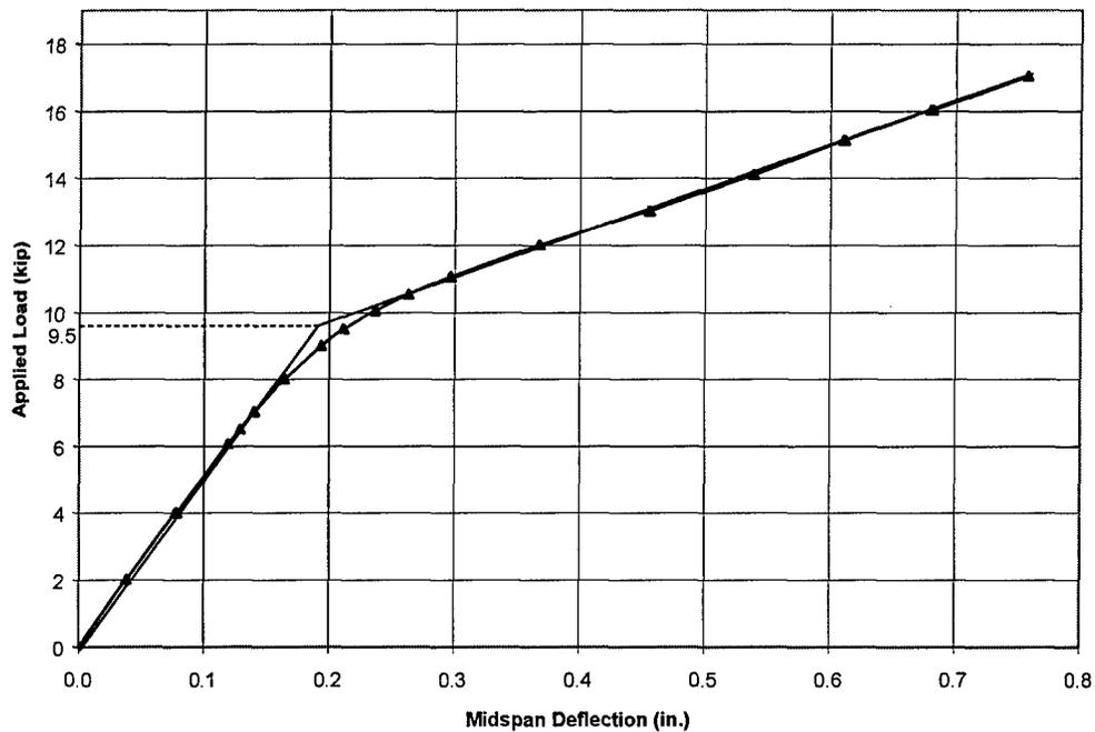
**Figure 4-3 Estimated Decompression Load Using Midspan Deflection—Beam 4**
