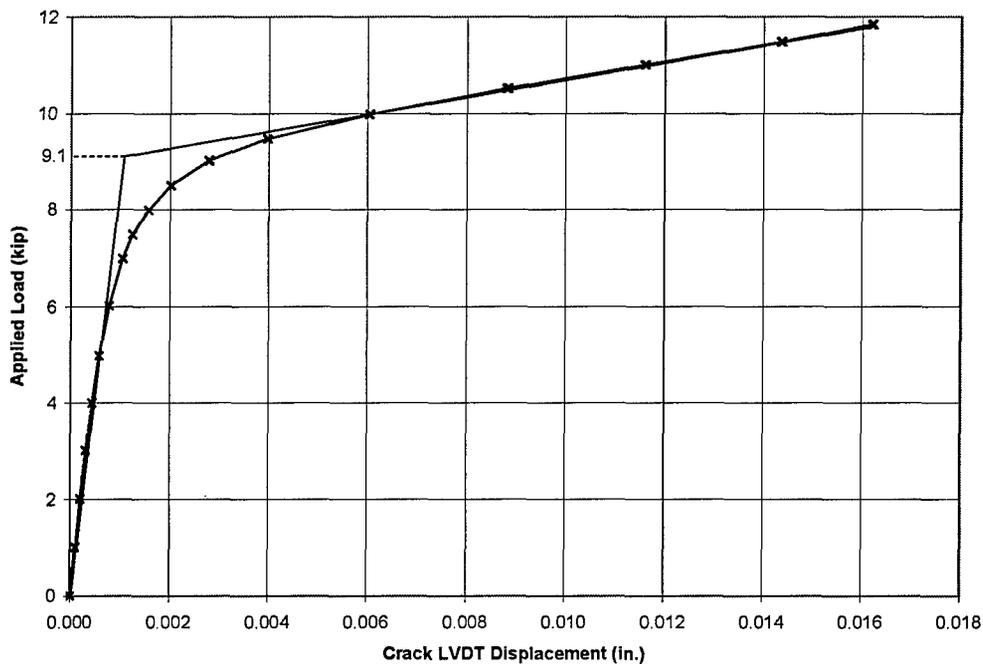
**Figure 4-37 Estimated Decompression Load Using Crack LVDT Displacement—Beam 3**
