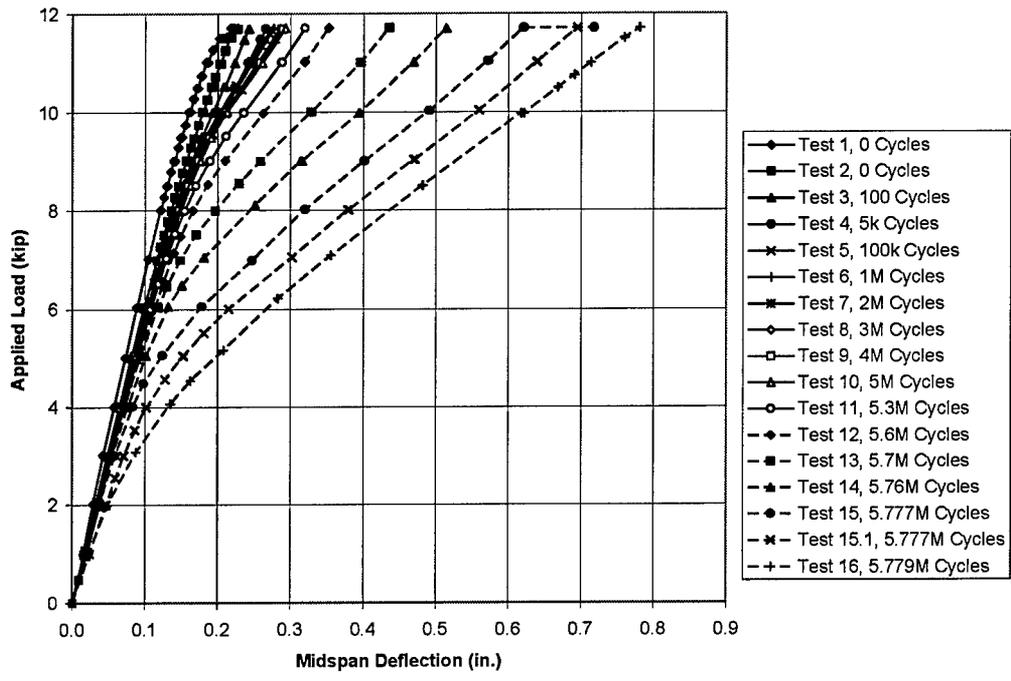
**Figure 4-55 Variation of Midspan Deflection During Fatigue Tests—Beam 2**
