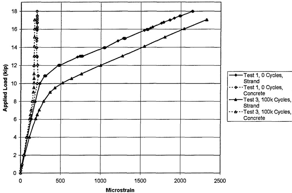
**Figure 4-8 Comparison of Strand Strain and Concrete Strain—Beam 4**
