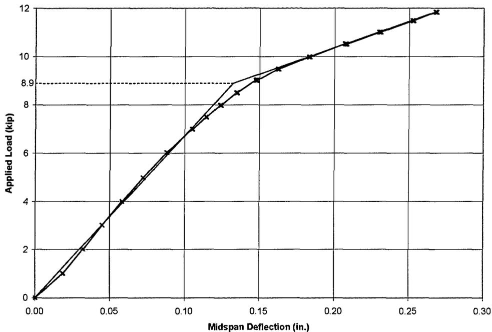
**Figure 4-36 Estimated Decompression Load Using Midspan Deflection—Beam 5**
