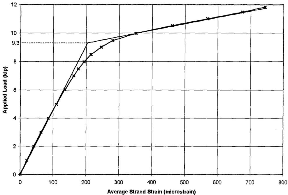
*Figure 4-35 Estimated Decompression Load Using Average Strand Strain—
