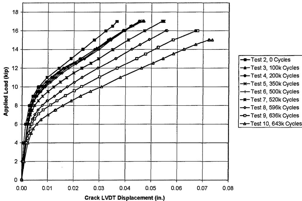
**Figure 4-9 Variation of Crack Gage Displacement During Fatigue Tests—
