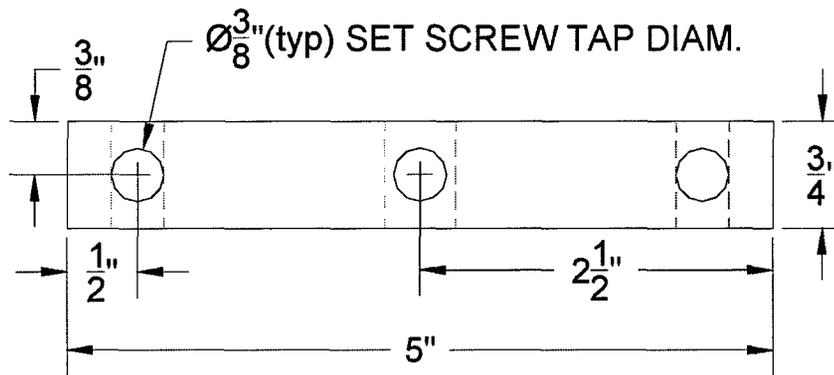
*Figure C-4 Front View of Top Aluminum Block*
