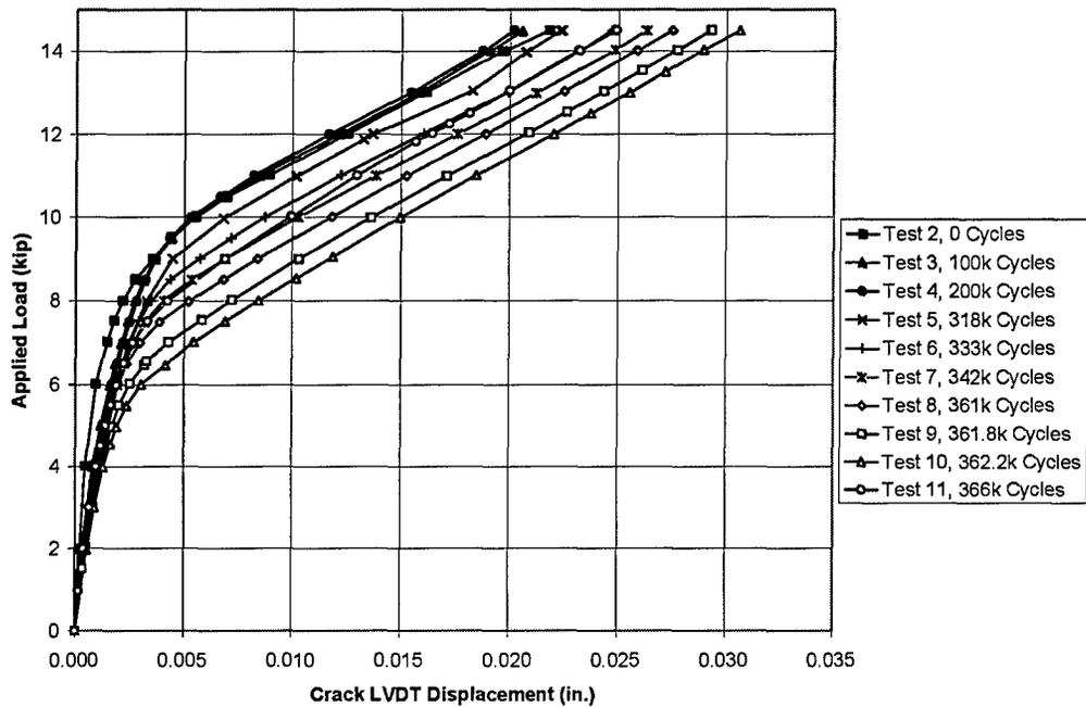
**Figure 4-26 Variation of Crack Gage Displacement During Fatigue Tests—
