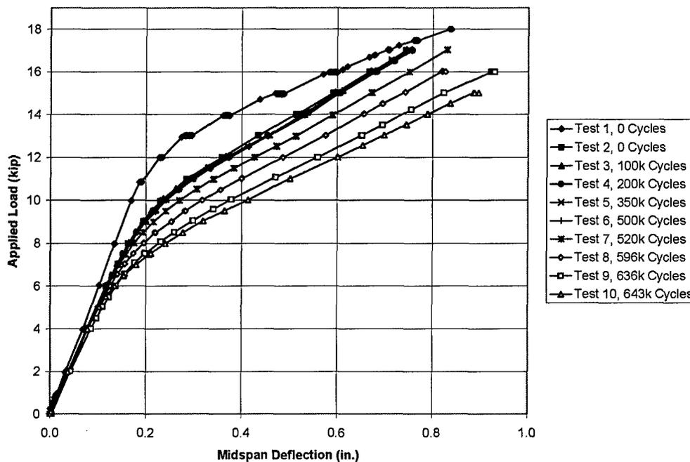
**Figure 4-5 Variation of Midspan Deflection During Fatigue Tests—Beam 4**
