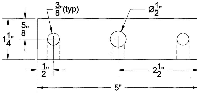
*Figure C-3 Top View of Top Aluminum Block*
