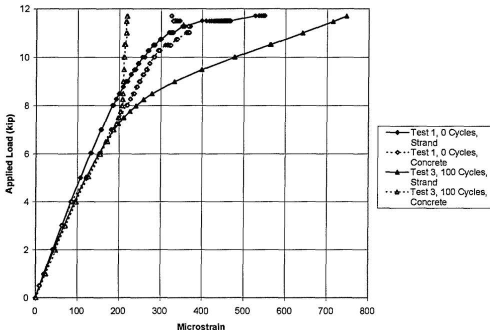
**Figure 4-59 Comparison of Strand Strain and Concrete Strain—Beam 2**
