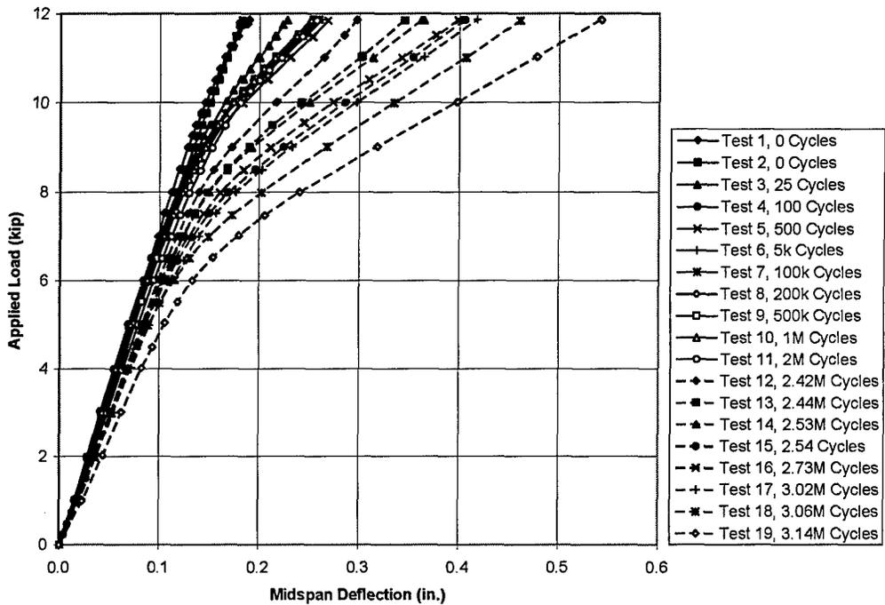
**Figure 4-38** Variation of Midspan Displacement During Fatigue Tests—Beam 3
