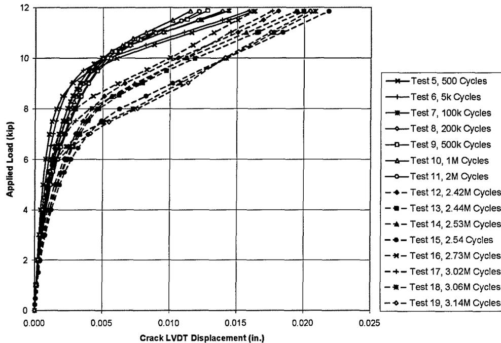
**Figure 4-43 Variation of Crack Gage Displacement During Fatigue Tests—
