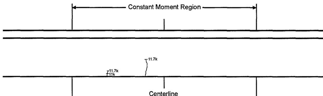
**Figure 4-51 Crack Pattern Following Initial Static Test—Beam 2**
