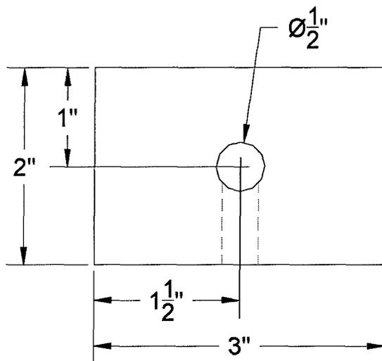
*Figure C-5 Top View of Middle Aluminum Block*
