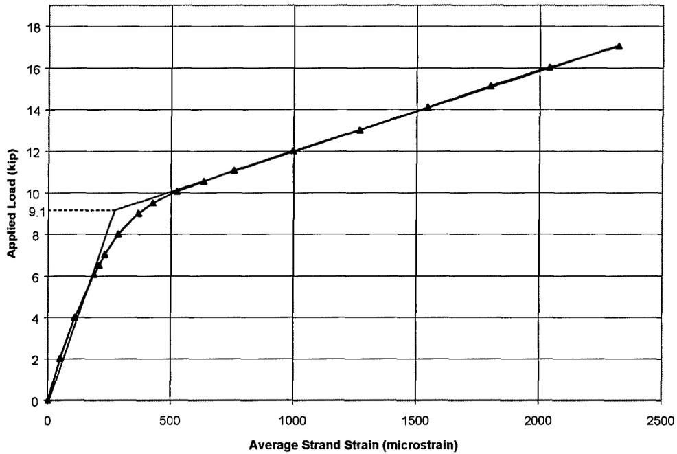
**Figure 4-2 Estimated Decompression Load Using Average Strand Strain—
