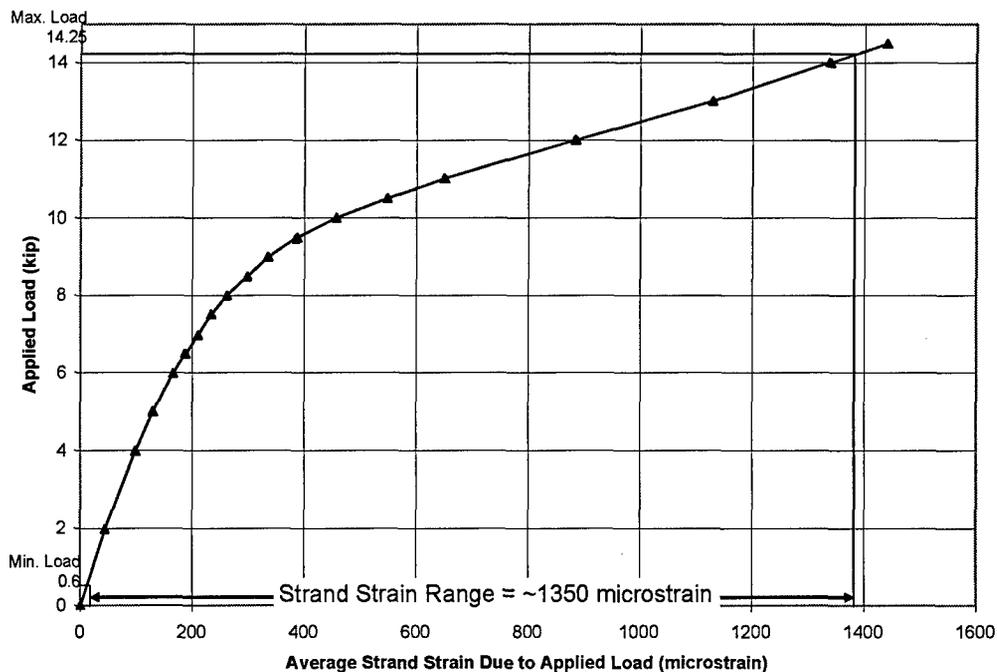
*Figure 5-1 Example of Determining Strand Strain Range--Beam 5*
