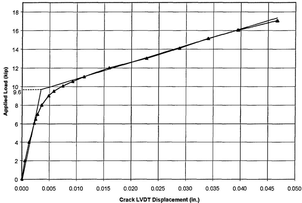
**Figure 4-4 Estimated Decompression Load Using Crack LVDT Displacement—Beam 4**
