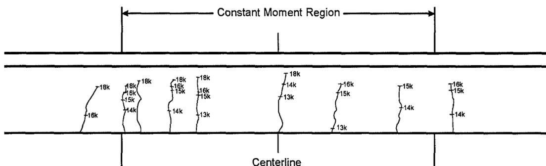
**Figure 4-1 Crack Pattern Following Initial Static Test—Beam 4**
