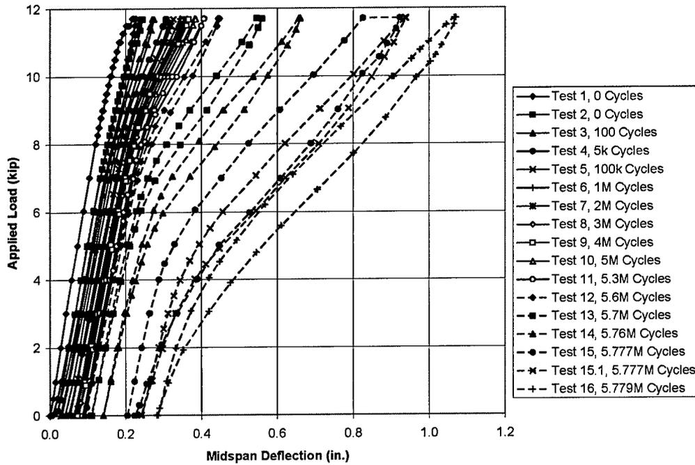
**Figure 4-56 Variation of Midspan Displacement, Including Permanent Offset—Beam 2**
