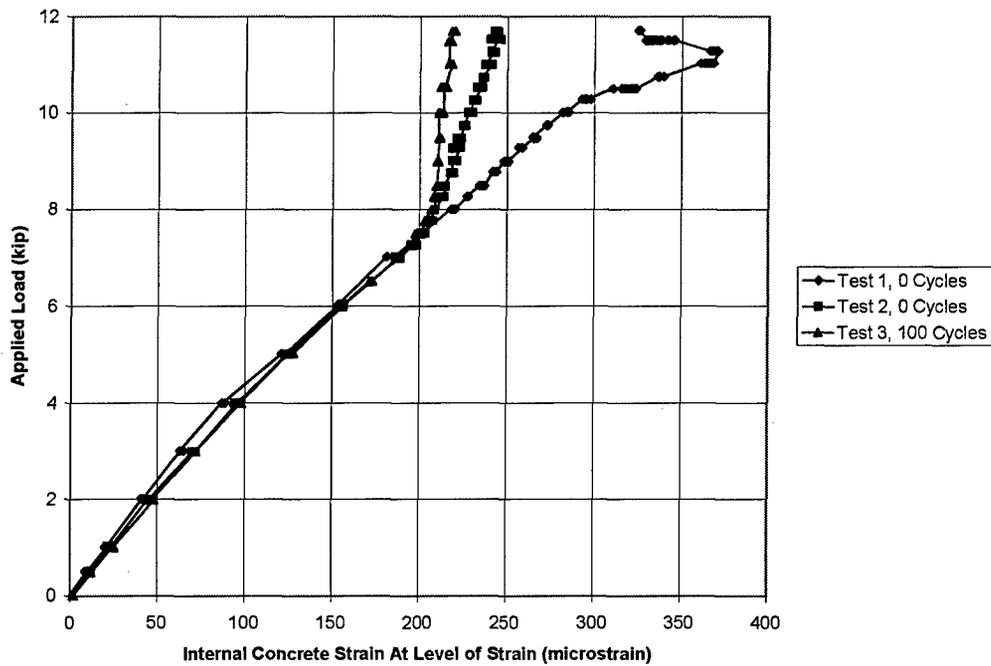
**Figure 4-58 Variation of Embedded Concrete Strain During Fatigue Tests—
