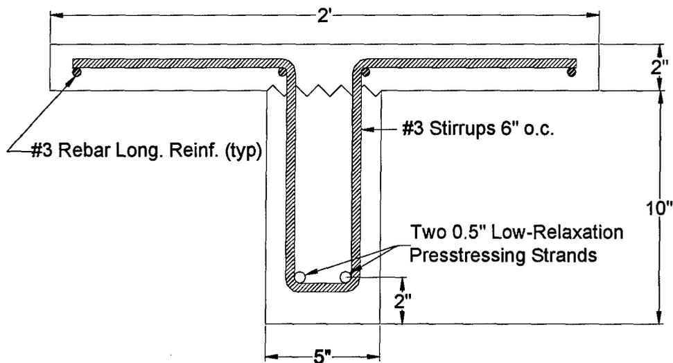
*Figure 3-1 Typical Beam Cross-Section*
