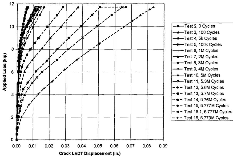
**Figure 4-60 Variation of Crack Gage Displacement During Fatigue Tests—
