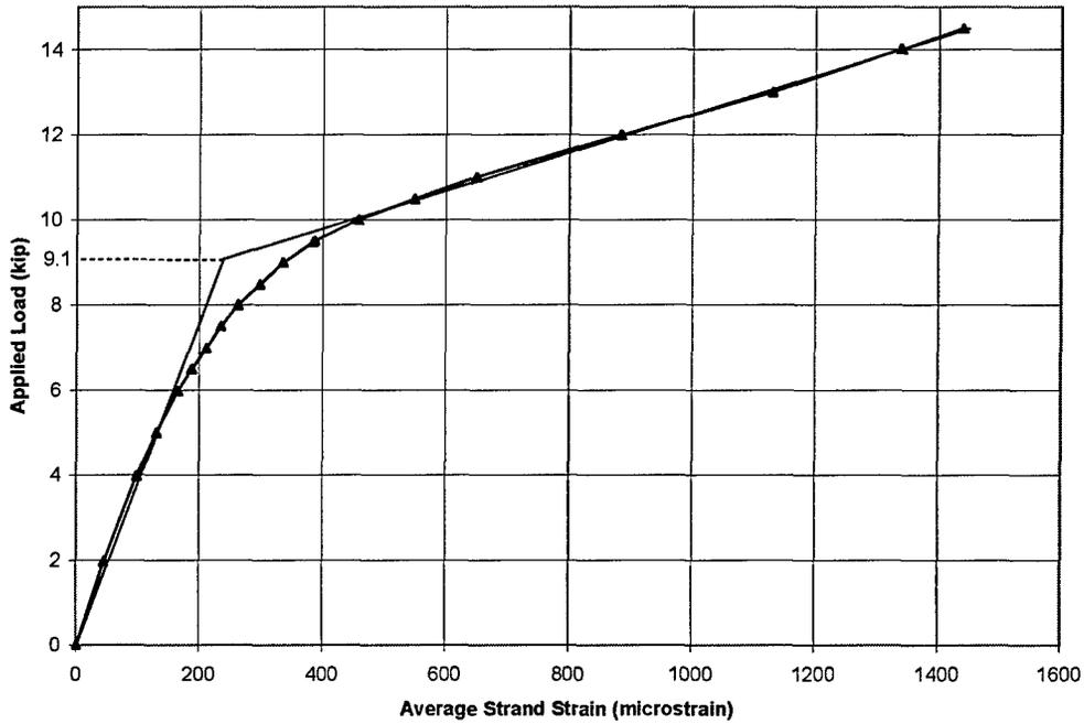
**Figure 4-18 Estimated Decompression Load Using Average Strand Strain—
