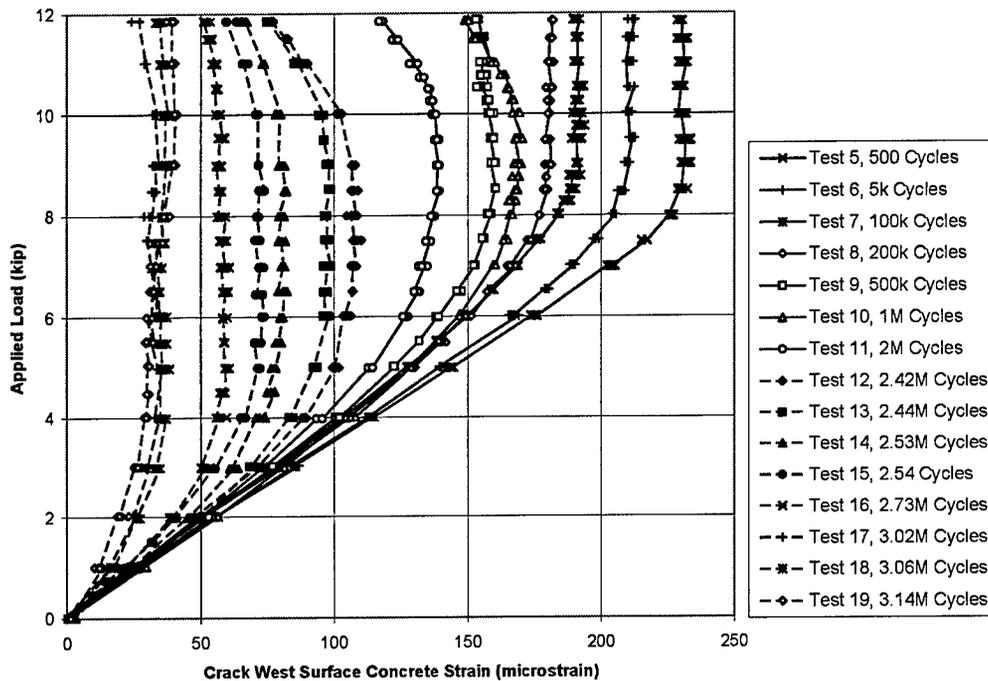
**Figure 4-45** *Variation of Concrete Surface Strain West of Crack During Fatigue Tests—Beam 3*
