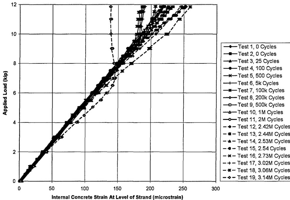
**Figure 4-41 Variation of Embedded Concrete Strain During Fatigue Tests—
