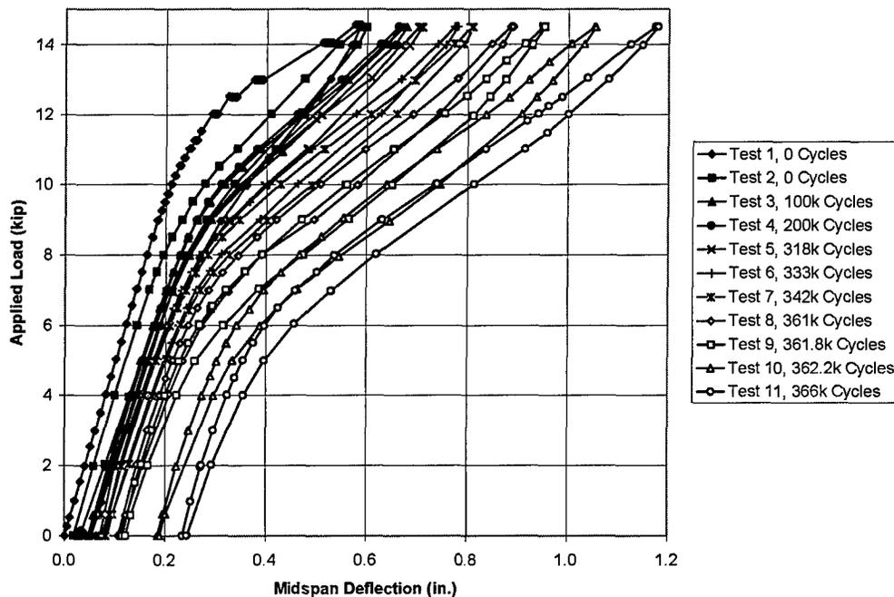
**Figure 4-22 Variation of Midspan Displacement, Including Permanent Offset—Beam 5**
