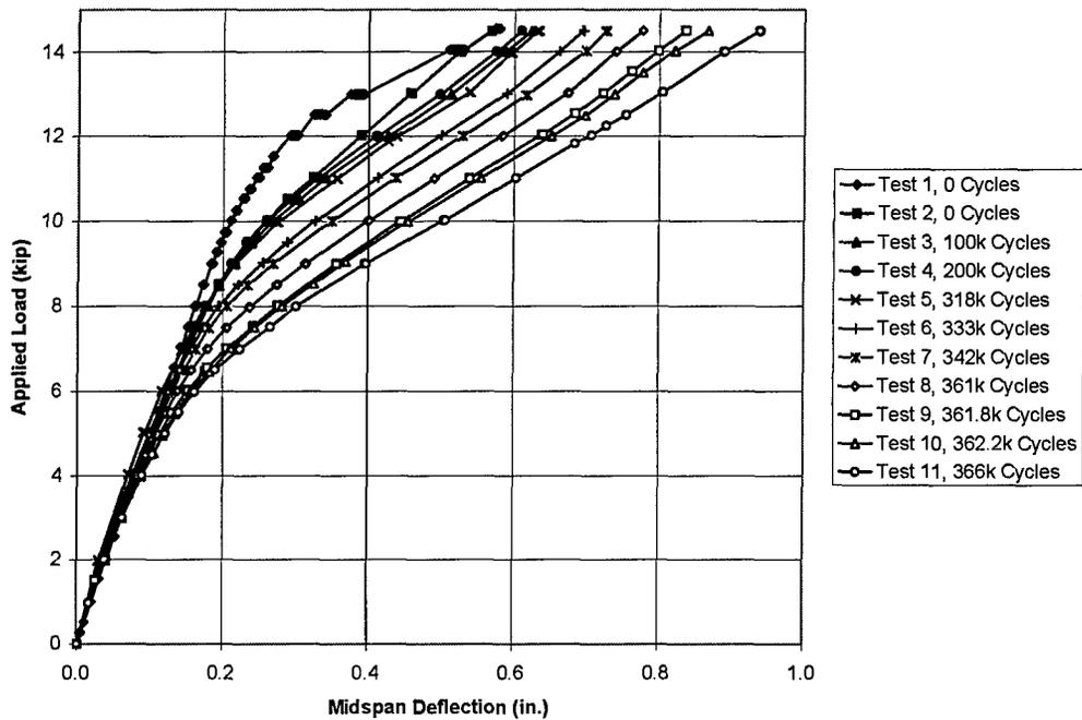
**Figure 4-21 Variation of Midspan Displacement During Fatigue Tests—Beam 5**
