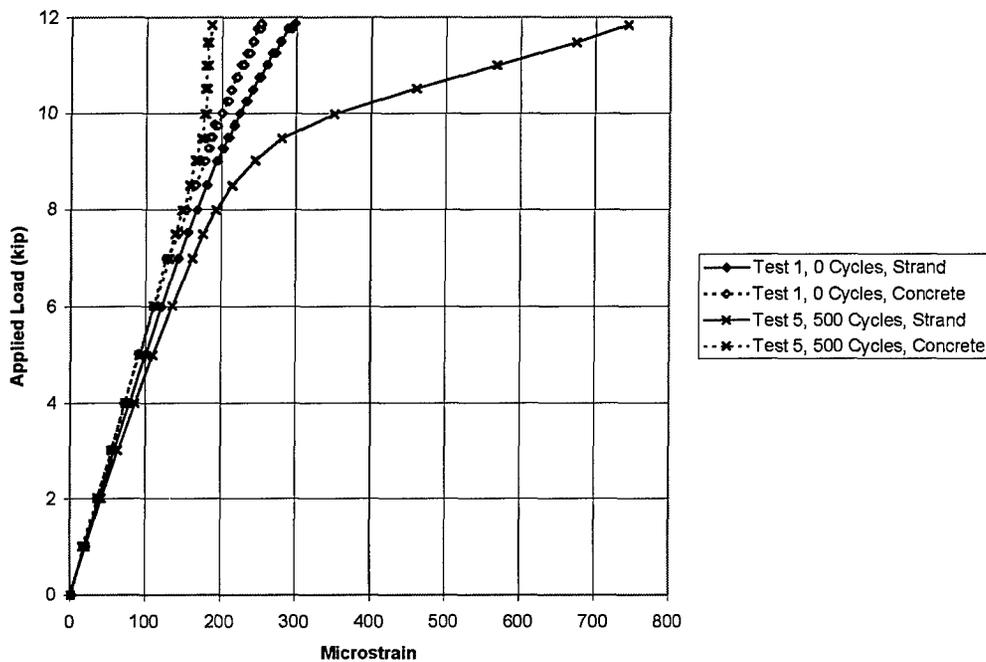
**Figure 4-42 Comparison of Strand Strain and Concrete Strain—Beam 3**
