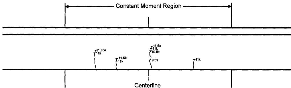
**Figure 4-34 Crack Pattern Following Third Static Test—Beam 3**
