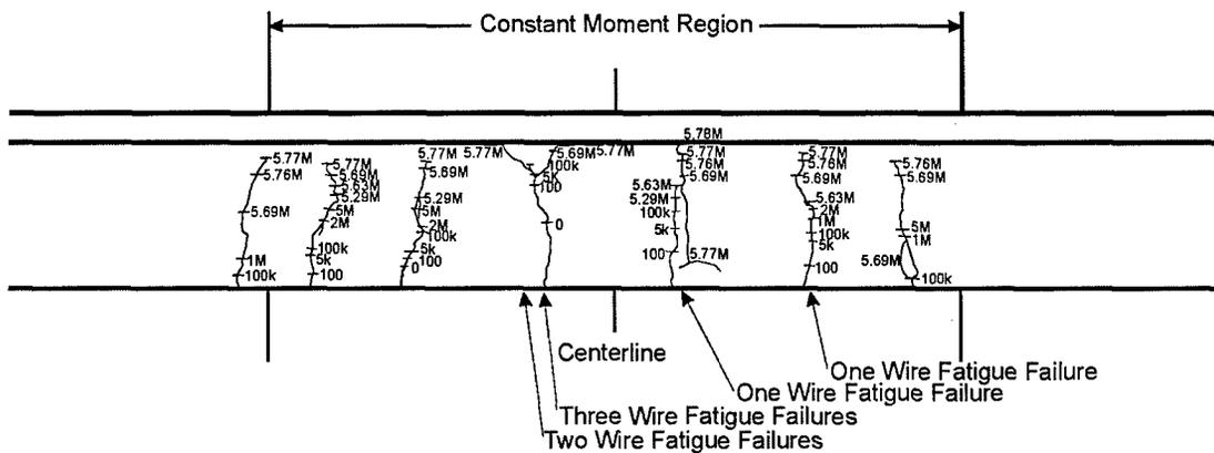
**Figure 4-67** Location of Wire Failures—Beam 2
