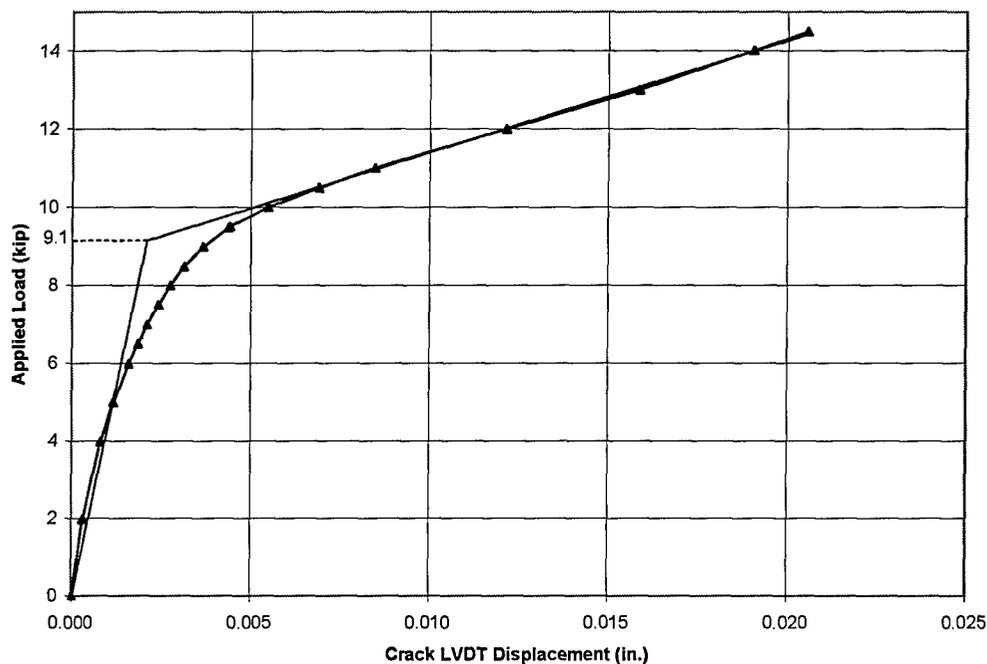
**Figure 4-20 Estimated Decompression Load Using Crack LVDT Displacement—Beam 5**
