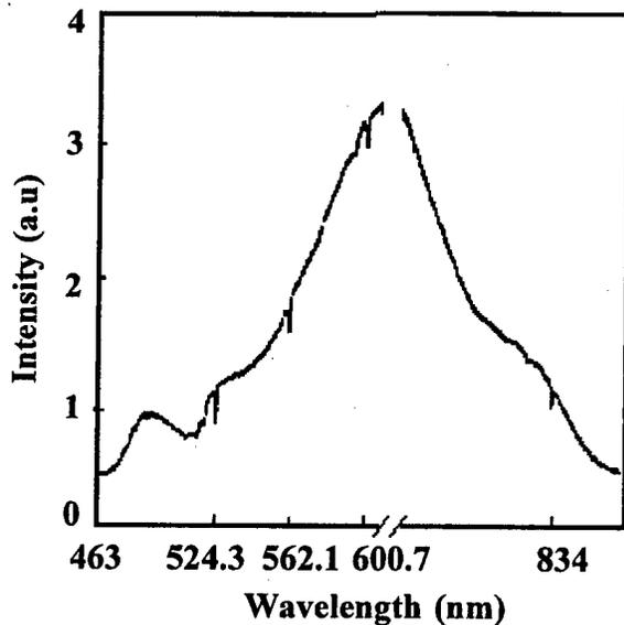
Fig. 3. Transmission spectrum of LiF color centers. Sharp lines at 834, 600.7, 562.1 and 524.3 nm are the ZPLs. Sample temperature was maintained at 10 K.
