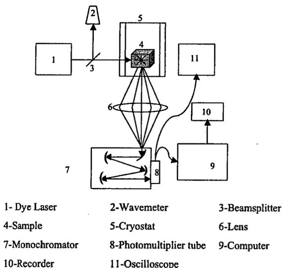
Fig. 1. Block diagram of the experimental setup.
