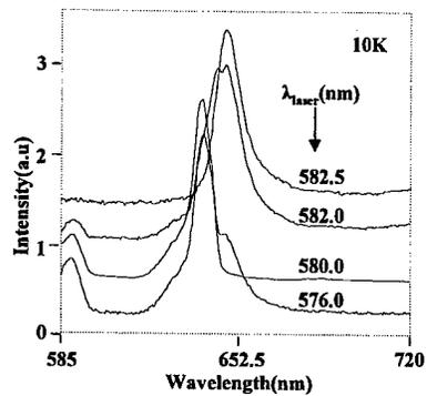
Fluorescence Spectrum of Eu<sup>3+</sup> as a function of laser excitation wavelength.
