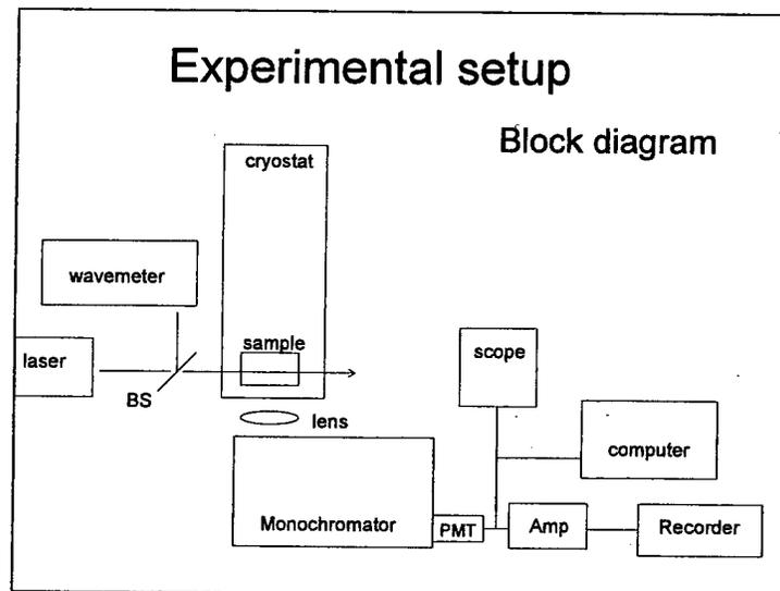
hole. A high power beam (typical power is 100mW) was used to burn a hole and a low power beam (~1mW) was used to probe the hole. A computer controlled medium
