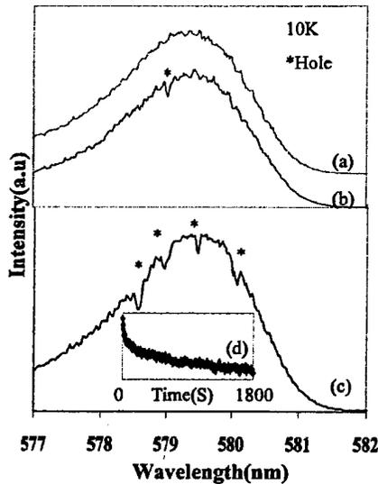
FIG. 1. Low temperature excitation spectrum of 612 nm emission before (a) and after (b) hole burning observed in  $\text{Eu}^{3+}$ -doped sodium borate glass. (c) Multiple hole burning in  $\text{Eu}^{3+}$ ,  $\text{Y}^{3+}$  codoped glass. Inset (d) shows emission intensity vs time during the hole formation, observed in  $\text{Eu}^{3+}$ ,  $\text{Y}^{3+}$  codoped sample.
