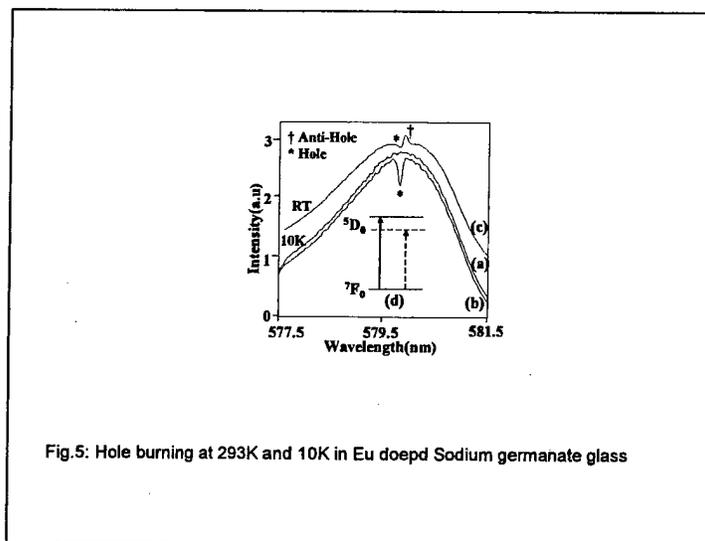
Fig.5: Hole burning at 293K and 10K in Eu doped Sodium germanate glass
