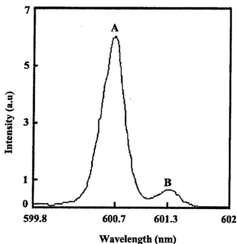
Fig. 5. Excitation spectrum of LiF reveals two sharp peaks (ZPLs) at 600.7 and 601.3 nm (peaks A and B). Fluorescence at 645 nm was monitored to record the spectrum. The sample temperature was maintained at 10 K.
