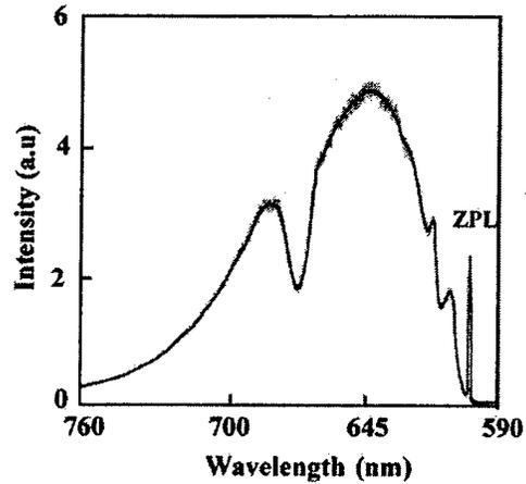
Fig. 4. Fluorescence spectrum of the sample reveals a sharp ZPL at 601 nm. The sample temperature was maintained at 10 K. The broad dip at 670 nm is due to a grating defect.
