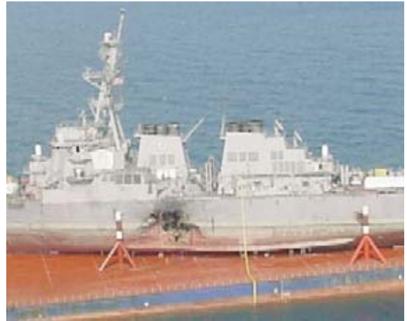
Figure 6: USS COLE damage xxxix
