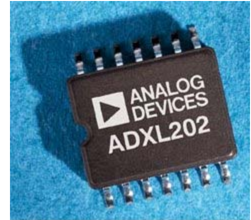
Figure 6. iMEMS accelerometer in surface mount package
