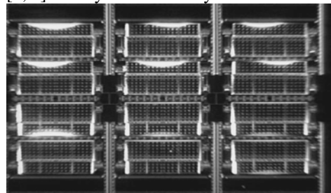
Fig.1: Optical image of louver array, with louvers all in closed position.
