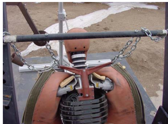
Figure 26: Details of a Special Bracket made to Support the Hybrid III Mannequin. (Picture Courtesy of DRDC, Canada)
