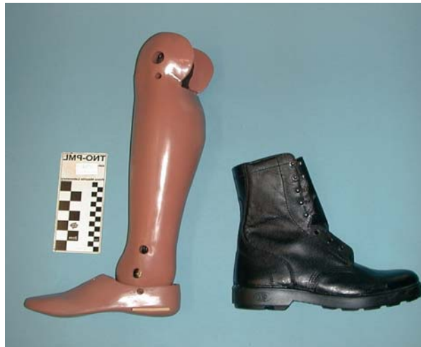
Figure 14: The Netherlands Mechanical Leg. (Picture Courtesy of TNO PML, Netherlands)
