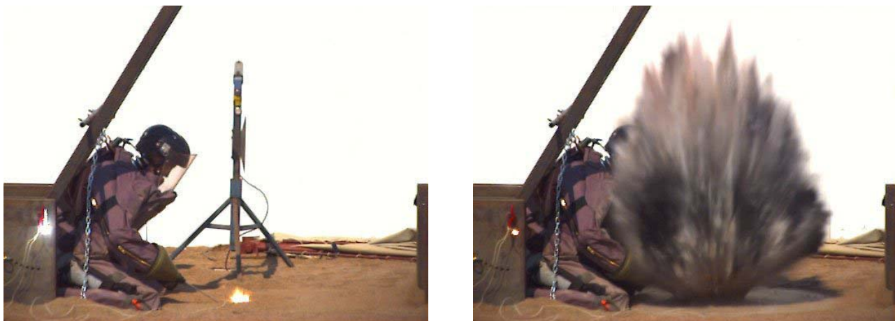
Figure 11: Explosion of a C4 Mine Surrogate Buried under 20mm of Sand showing the Loading Zone on a Mannequin Dressed with Protective Ensemble; timing between frames is 1msec; note the glow at upper edge of the detonation products indicating continued burning of case fragments. (Pictures courtesy of DRDC, Canada)
