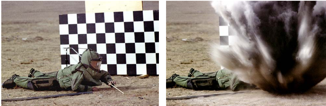
Figure 10: PMA-1 Mine Explosion showing the Loading Zone on a Mannequin Dressed with a Protective Ensemble. (Pictures Courtesy of DRDC, Canada)
