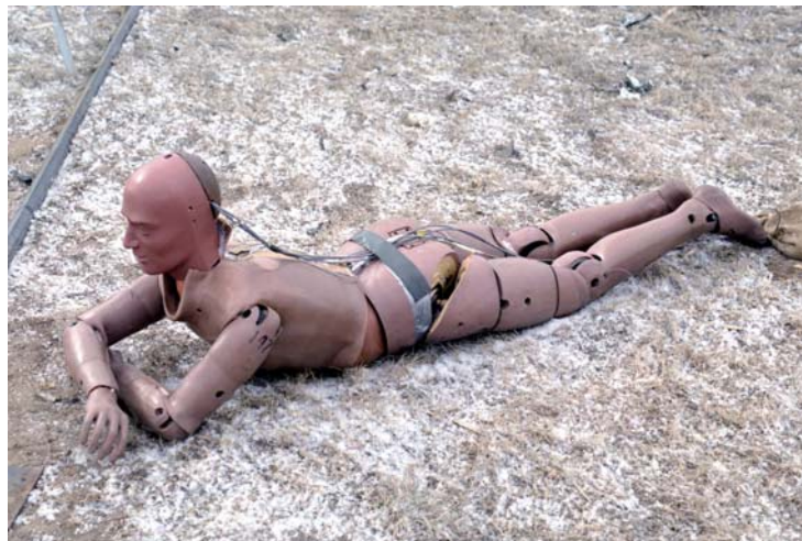
Figure 29: Discarded Hybrid II Mannequin with Modified Neck. (Picture Courtesy of DRDC, Canada)
