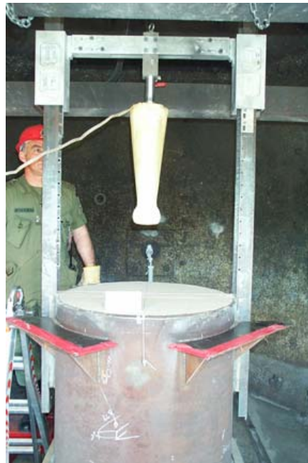
Figure 22: Test Rig for Lower Limb Surrogate Testing and PPE Evaluation. (Picture Courtesy of DRDC, Canada)
