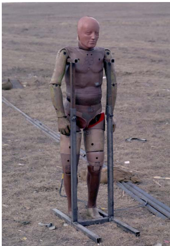
Figure 28: Crutches Type Support Rig for Fragmentation Tests. (Picture Courtesy of DRDC, Canada)
