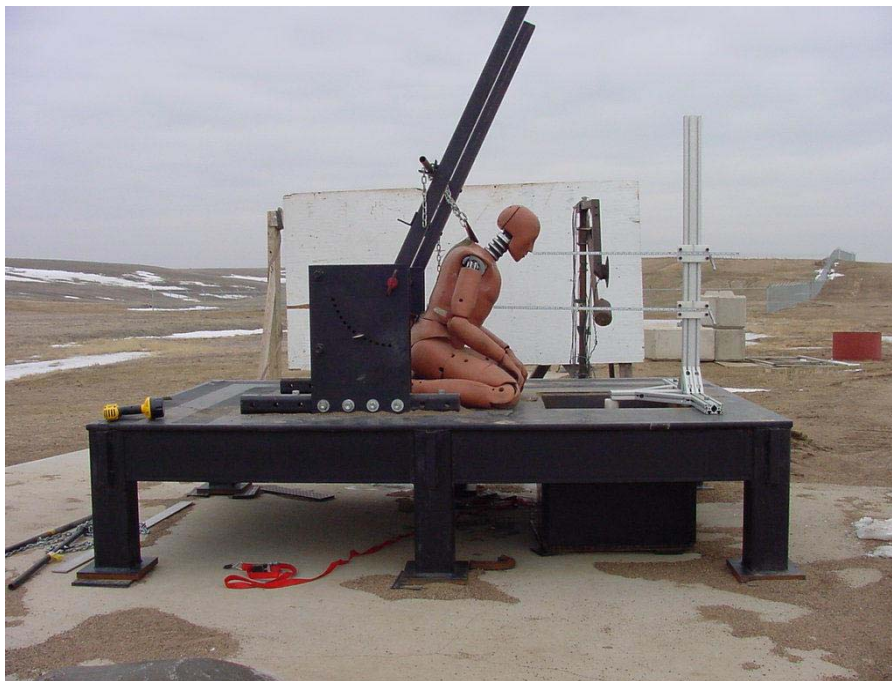
Figure 27: Rigid Test Platform with Positioning Rig and Measurement System. (Picture Courtesy of DRDC, Canada)
