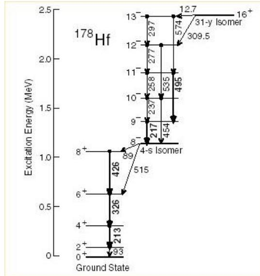
Figure 1. Energy Level Diagram of  $^{178}\text{Hf}^{m2}$  Decay (13)
