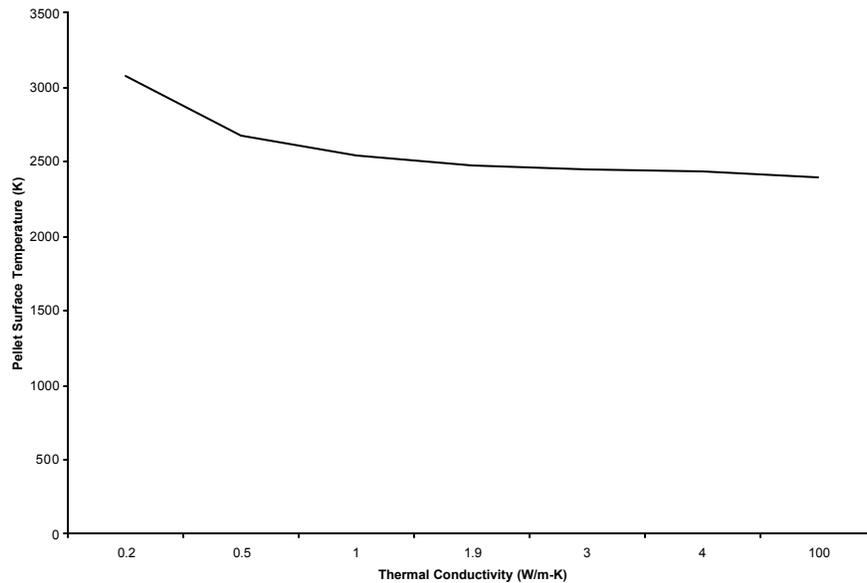
Figure 10. Effect of Thermal Conductivity on Propellant Temperature
