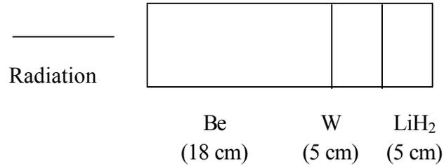
Figure 6. Typical Fission Reactor Shadow Shield (3:496)
