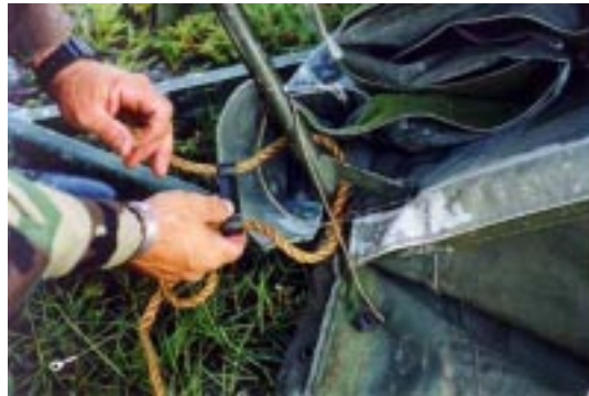
Figure 26. Attachment of Guy Ropes to Eave and Ridge Extenders.
