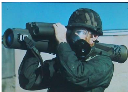
Figure V-5. An Early Mockup of the Shoulder Fired Tankbreaker and the Key to Its Fire and Forget Capability—the Staring Thermal Imaging Seeker (Right)
