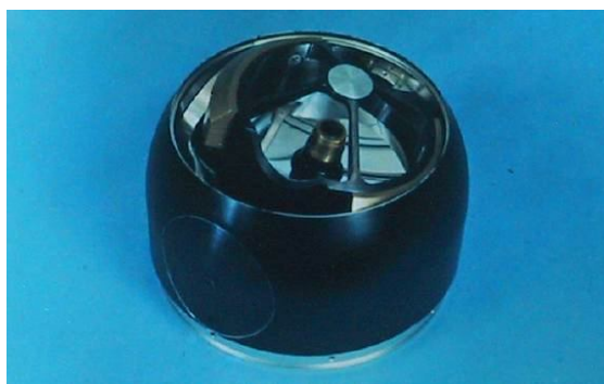
Figure V-5. An Early Mockup of the Shoulder Fired Tankbreaker and the Key to Its Fire and Forget Capability—the Staring Thermal Imaging Seeker (Right)
