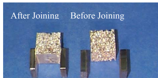
Figure 66. Double lap shear (DLS) specimen before and after joining
