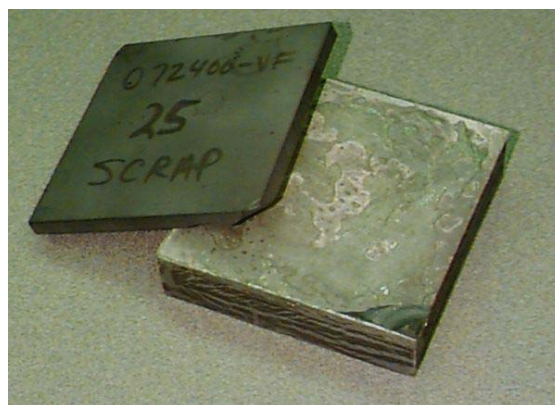
Figure 72. 4x4 inch ballistic test sample shown in Figure 2, after CTE mismatch led to bond failure (2 days elapsed time).
