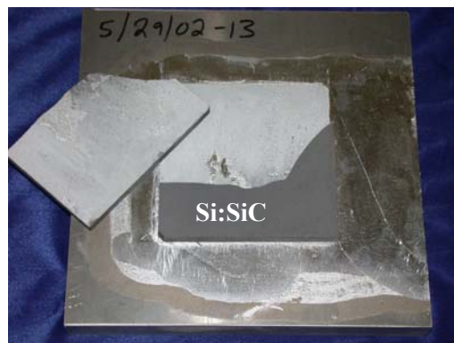
Figure 81. Si:SiC plate S-Bond™ 400 joined directly to 3/4" aluminum plate partially on bonded side.
