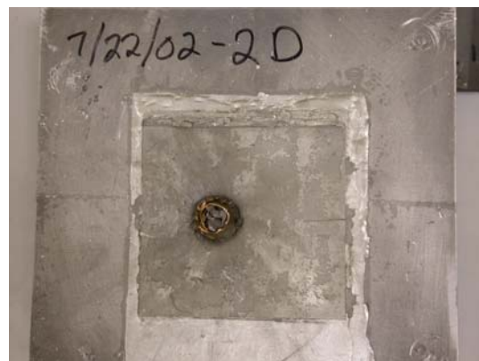
Figure 85 – Plate 2D – (SiC tile w/ mechanical activation and an Al:SiC intermediate layer) – The strike velocity was nearest the 2171 fps constructed V50.
