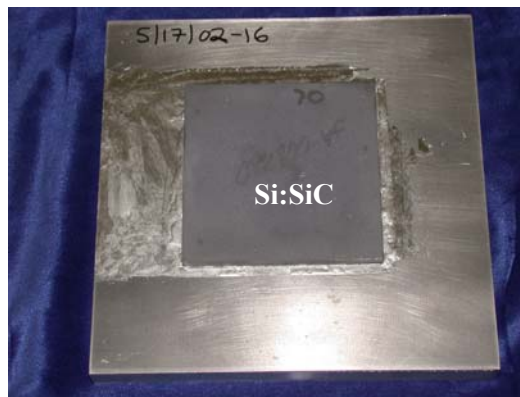
Figure 77. Si:SiC composite plate S-Bond™ 220 joined directly to 3/4" aluminum plate
