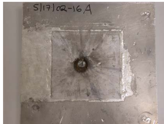
Figure 89 – Plate 16D (Si:SiC composite tile vacuum pretreated with S-Bond 220 paste) – The strike velocity was nearest the 2243 fps constructed V50
