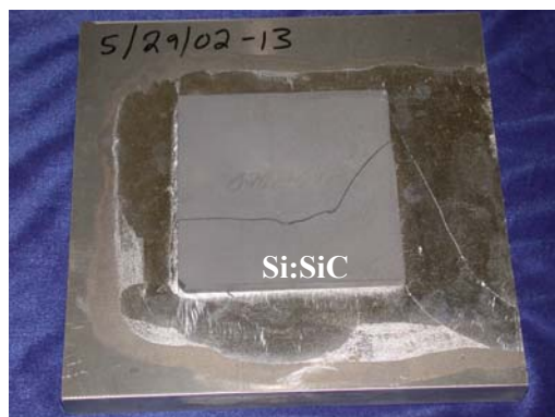
Figure 80. Si:SiC plate S-Bond™ 400 joined directly to 3/4" aluminum plate.
