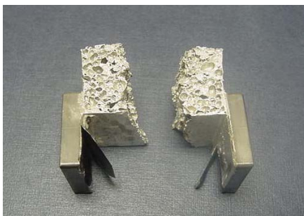
Figure 67 and 68. Pictures of failed composite armor test samples.
