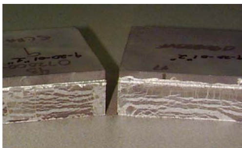
Figure 75. Macro view of Al:SiC transition piece / S-Bond™ joined composite armor plates
