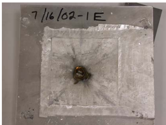
Figure 84 – Plate 1E (SiC tile w/ mechanical activation only) – The strike velocity was nearest the 2160 fps constructed V50.
