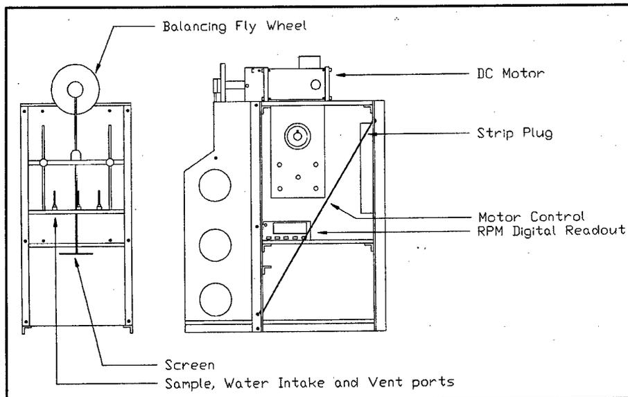
Figure 2. Schematic of the Particle Entrainment Simulator (PES)
