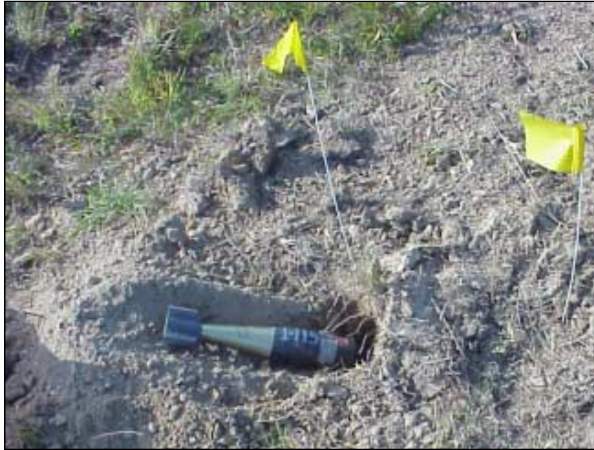
Figure N-6. UXO placement for burial.
