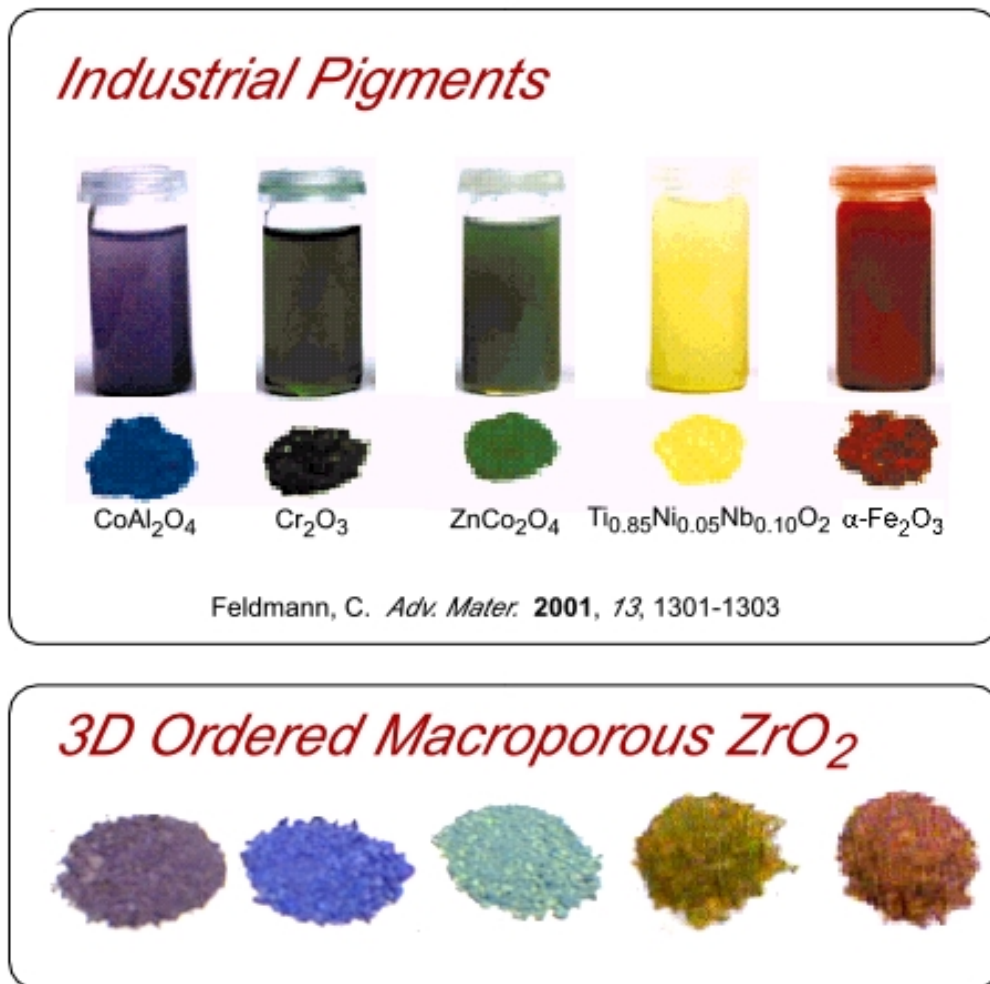
Figure 8. Colors of 3DOM \text{ZrO}_2 compared to industrial pigments. The three 3DOM \text{ZrO}_2 samples on the bottom left have increasingly larger pore sizes. The pore sizes depend on the size of the PMMA latex spheres used as templates. The two samples on the right correspond to the first two, filled with ethanol.
