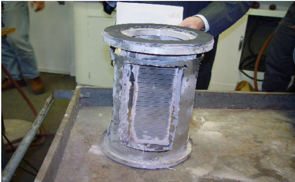
FIGURE 2. SIDE VIEW OF MOF FILTER #1 PREFILTER CUT AWAY
