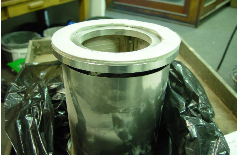
FIGURE 1. SIDE VIEW OF MOF FILTER #1 WITH PREFILTER
