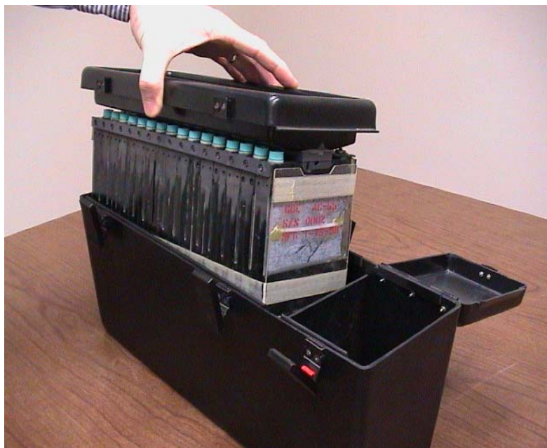
Figure 4 View of the SOFAL aluminum air battery unit. This unit is an aluminum air battery produced by the company. The SOFAL cells are stacked together inside the unit. The cells are about four inches across.
