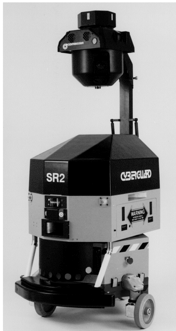
Figure 2. MDARS-I robotic platform based upon the Cybermotion K2A.
