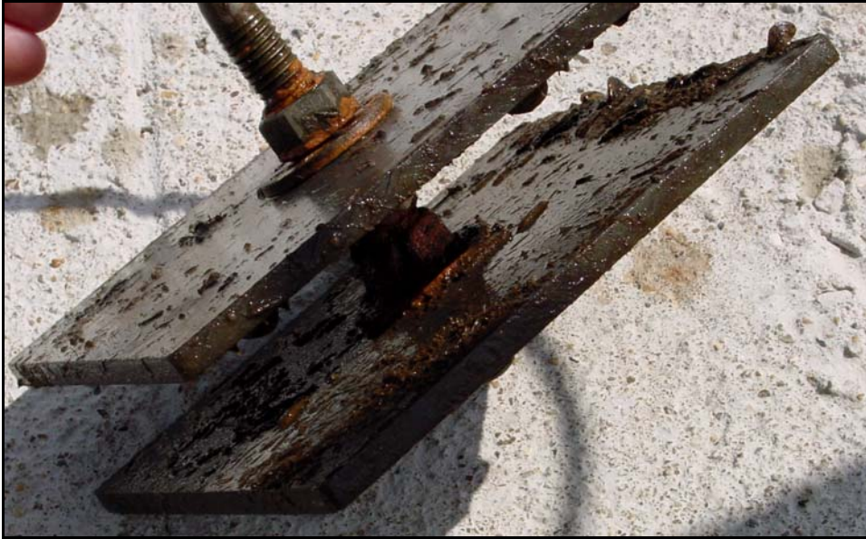
b. Set of small plates retrieved from the water, showing zebra mussels attached along the right-hand edge.
