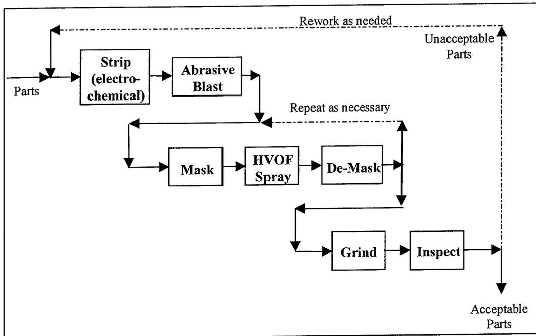
Figure 4-2. Process Flow of HVOF for Applying WC/Co
