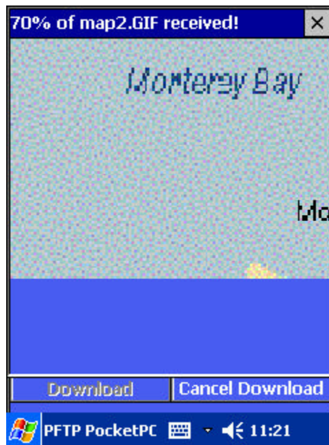
Figure 44. Paused state of the user interface after a connection loss (Pocket PC)
